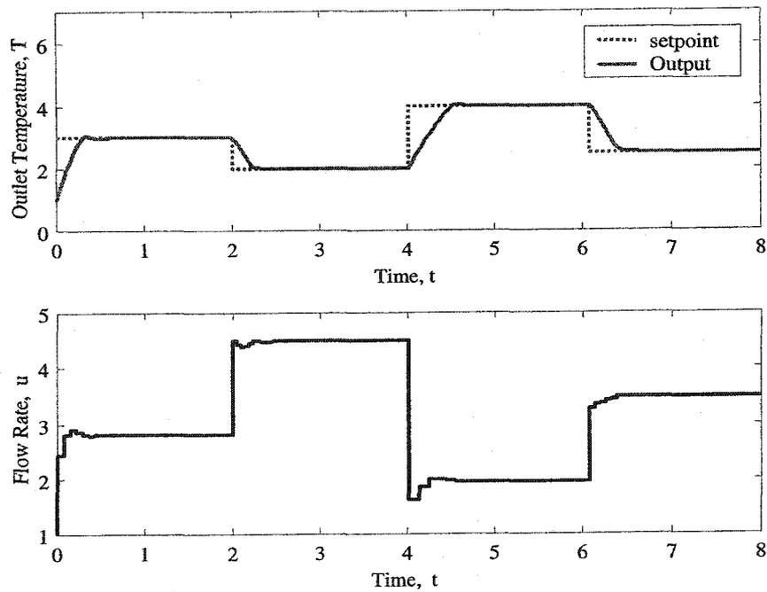
Figure 4.6: Setpoint tracking response of CBMPC in the heat exchanger
