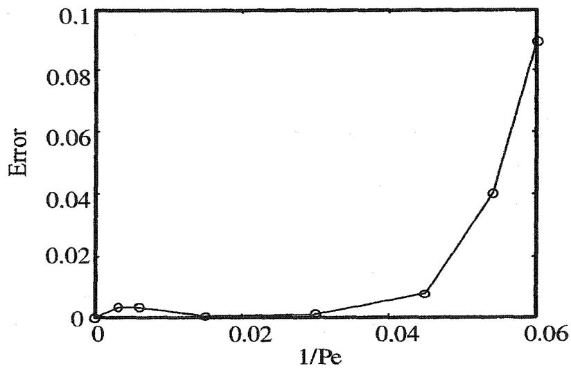
Figure 6.12: Output prediction error of CMCFD in the bleaching reactor
