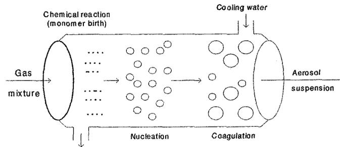
Figure 1.2: Aerosol flow reactor
