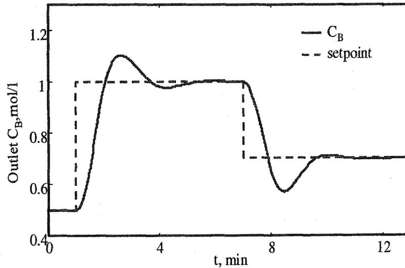
Figure 3.11: Output response to setpoint changes in PFR
