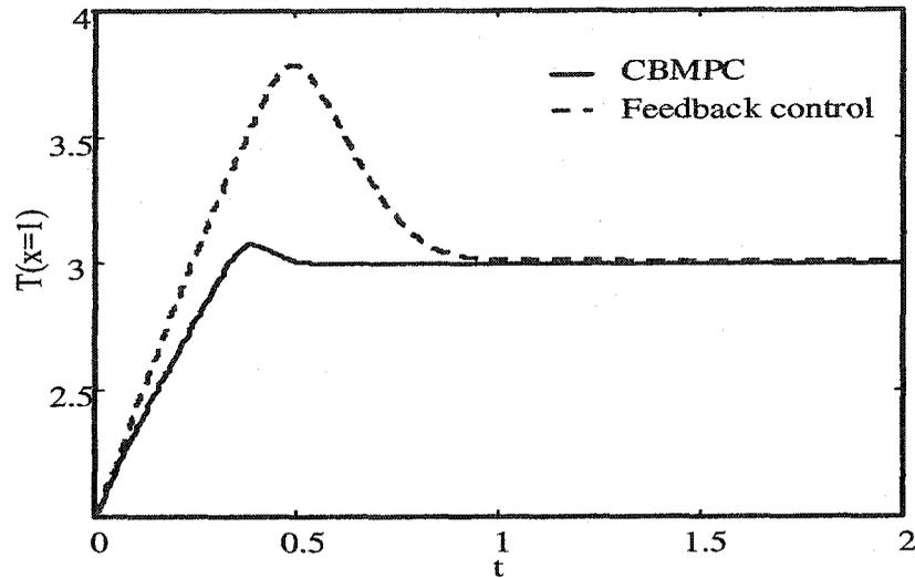
Figure 4.8: Performance comparison of CBMPC vs. standard feedback control
