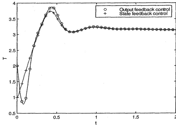
Figure 3.8: Comparison of temperature evolution at  $x=1$  by output feedback control vs. state feedback control in the heat exchanger
