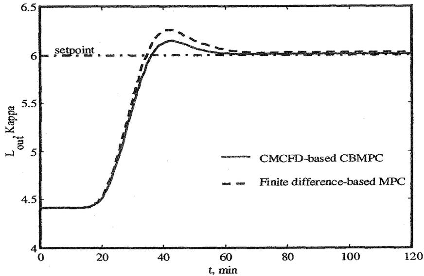
Figure 6.14: Comparison of CMCFD-based CBMPC vs. finite difference-based MPC
