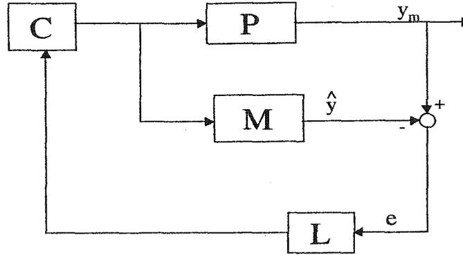
Figure 6.1: Structure of model-plant mismatch compensation in CBMPC
