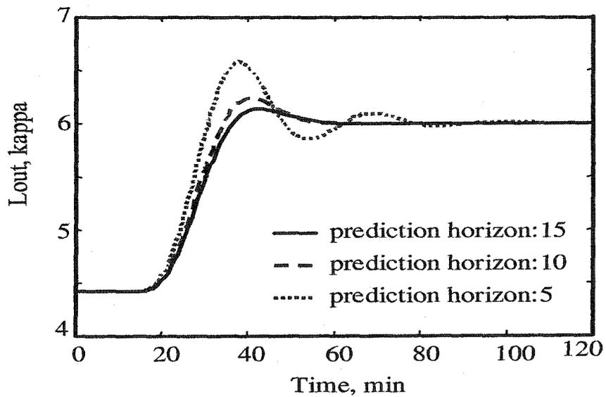
Figure 6.16: Output response of the CMCFD-based CBMPC for different prediction horizons
