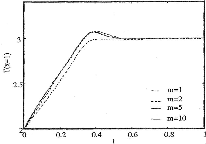
Figure 4.7: Output response of CBMPC for different discretizations in the heat-exchanger
