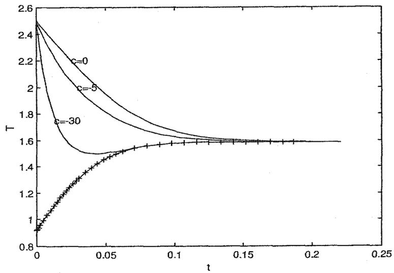
Figure 3.7: Comparison of true temperature evolution (+) vs. temperature evolution from the state observer at  $x=0.5$  in the heat exchanger
