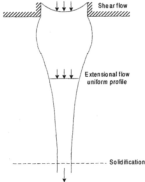
Figure 1.3: Melt spinning
