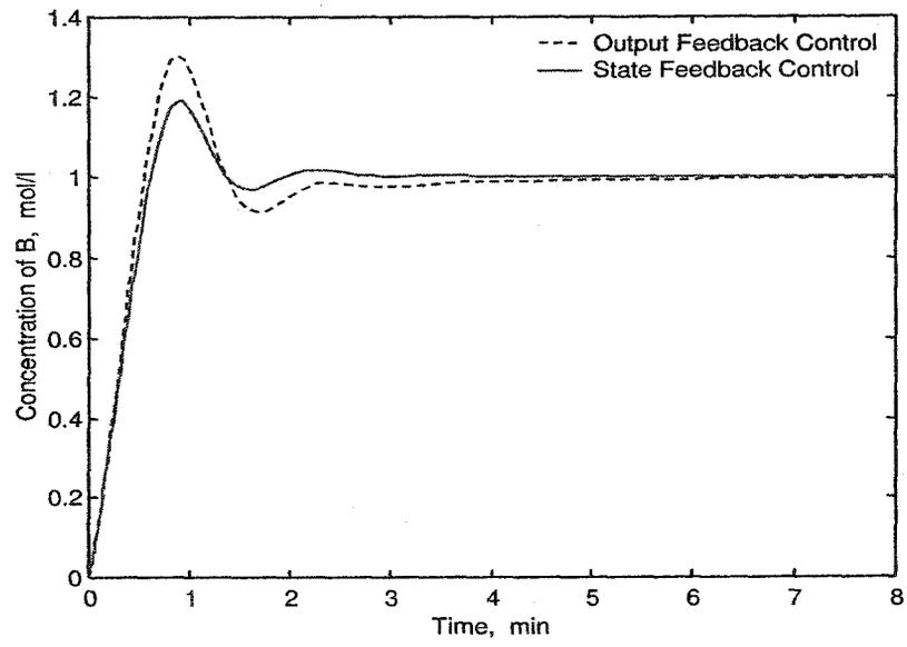
Figure 3.14: Comparison of state feedback control vs. output feedback control in PFR
