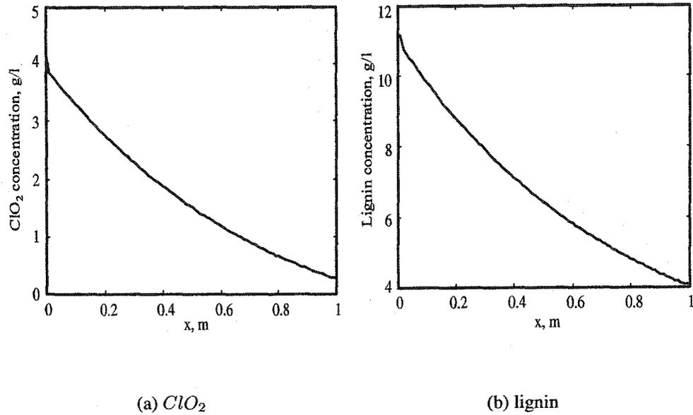
Figure 6.7: Initial profiles of the state variables in the MIMO bleaching reactor
