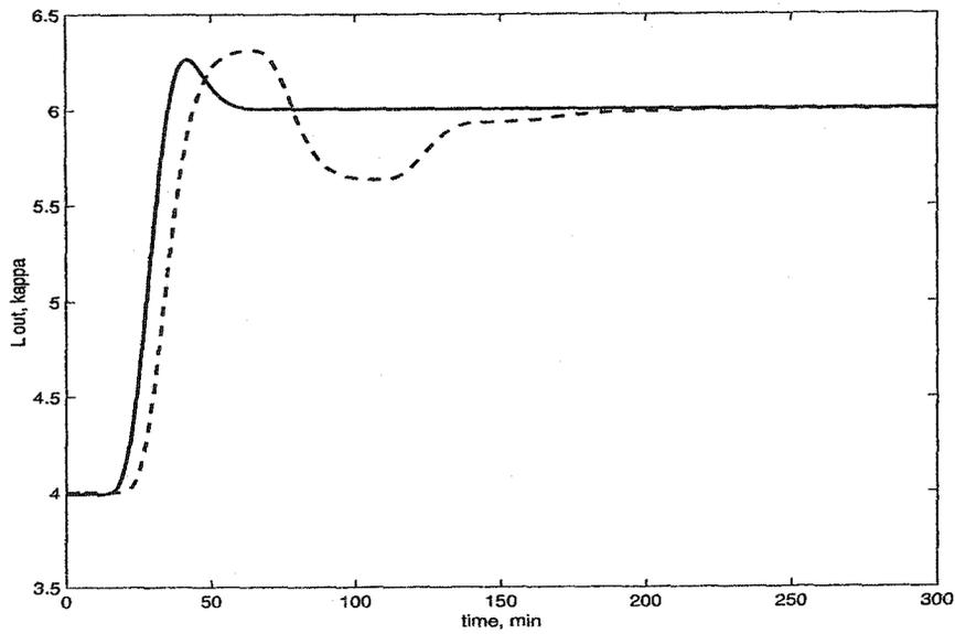
Figure 6.15: Comparison of CMCFD-based CBMPC vs. CBMPC with mismatch compensation
