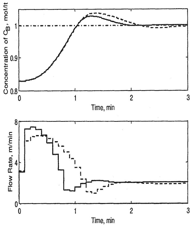
Figure 5.9: Performance comparison of CBMPC vs. finite difference-based MPC in the counter-flow PFR
