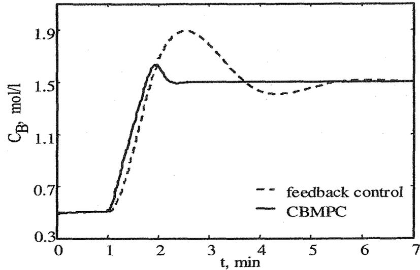
Figure 4.11: Performance comparison of the CBMPC and the state feedback control in PFR
