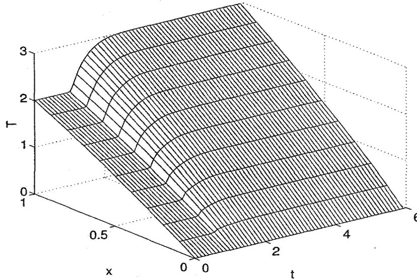
Figure 3.1: Setpoint tracking performance in the heat exchanger using state feedback
