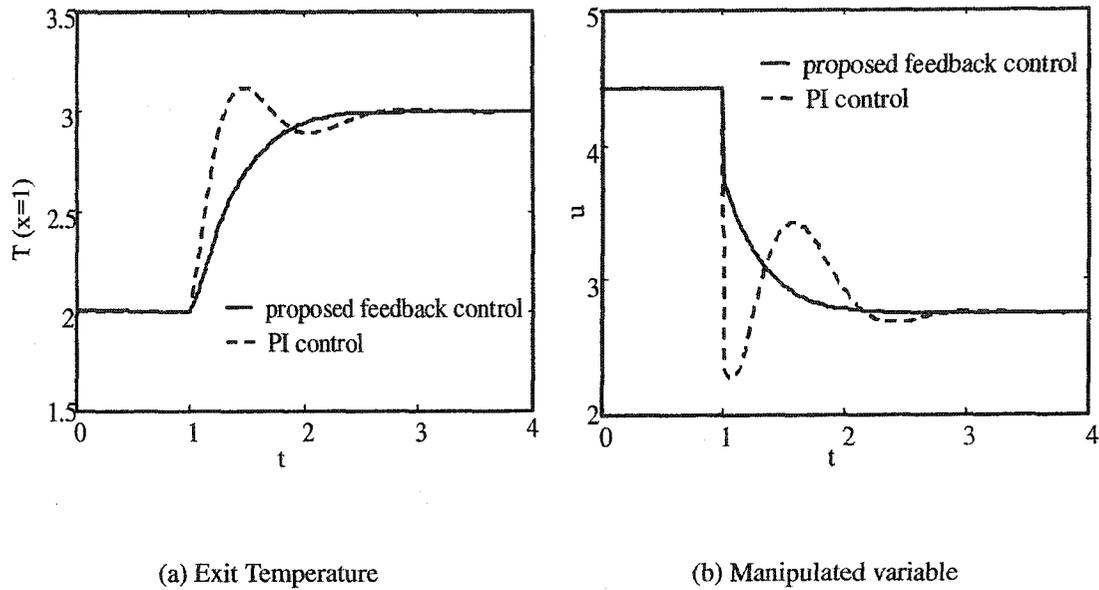
Figure 3.2: Comparison of the proposed state feedback vs. the conventional PI control
