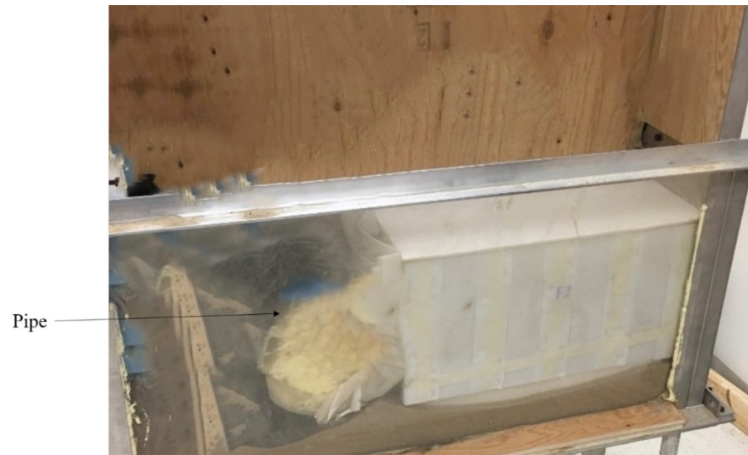
Figure 3- 4: a) Test setup components (horizontal loading shown); b) Pipe and the SGB assembly.
