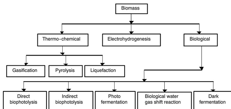
Figure 1. Biohydrogen production processes.
