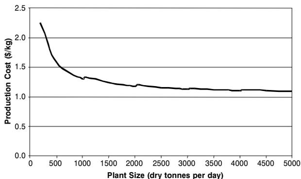
**Figure 5. Variation of H<sub>2</sub> production cost with plant size for whole-forest biomass.**
