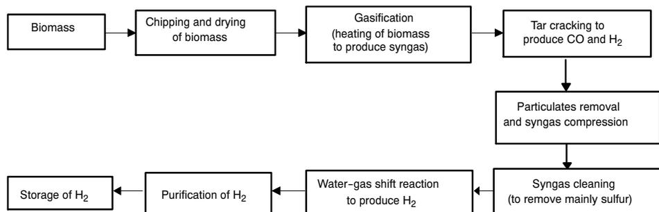
Figure 2. Hydrogen production from whole-forest biomass by gasification.
