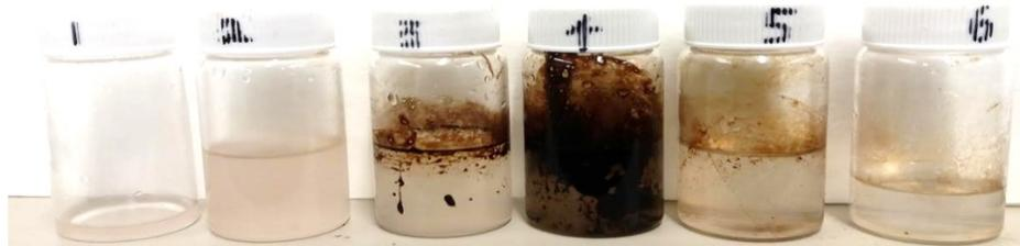
**Figure 17—Produced samples from low salinity water flooding at 1ml/min.**
