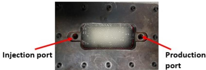
Figure 11—Top view of the glass bead model.
