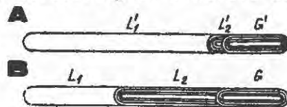
Fig. 87. Phase composition of syngenetic composite inclusions of \text{CO}_2 of homogeneous (A) and heterogeneous (B) trapping: L'1 , L'2 , G' and L1 , L2 , G - respectively volumes of water solution \text{LCO}_2 and gas.
