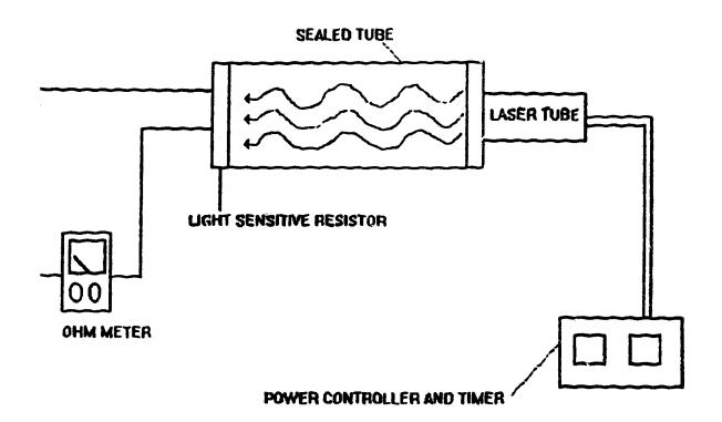
FIGURE 10: LASER CHECK CALIBRATION
