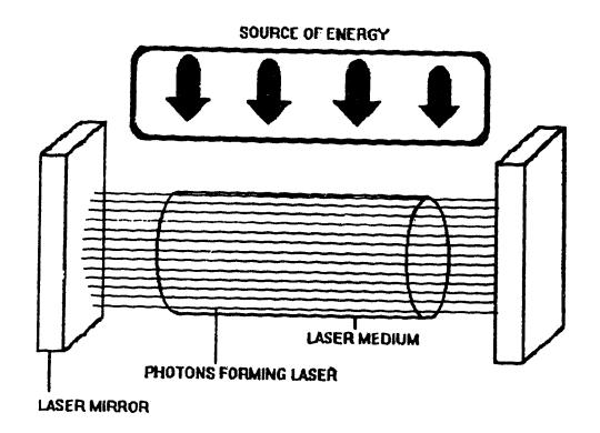
FIGURE 5: PHOTONS BUILD UP BECOMING INTENSE AND FORMING THE LASER
