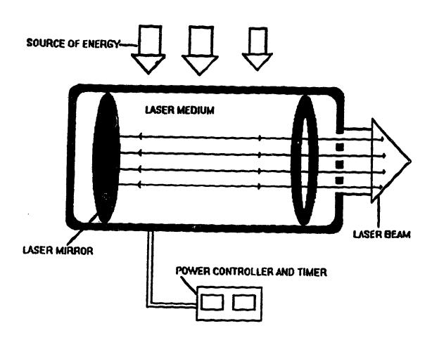
FIGURE 1: LASER SYSTEM WITH ITS PARTS
