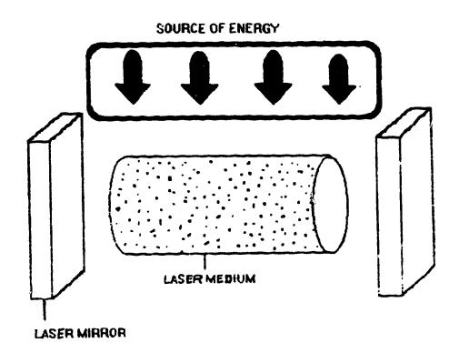
FIGURE 2: INTRODUCTION OF ENERGY INTO THE LASER MEDIUM
