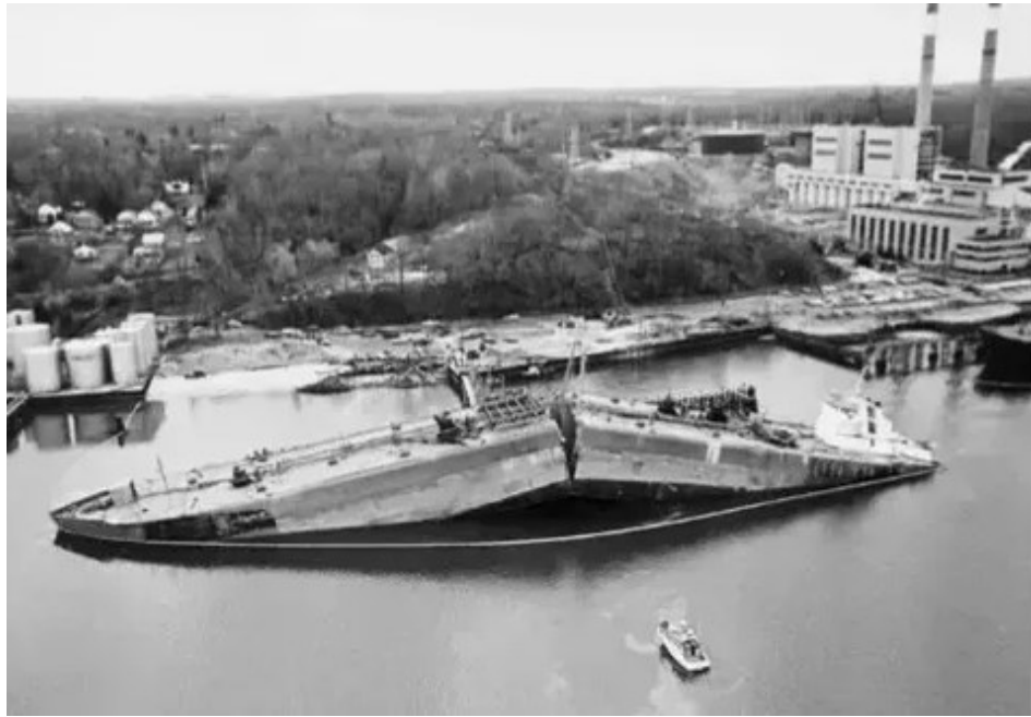
Figure 1 An oil tanker fractured by crack propagation around its girth [1] .
