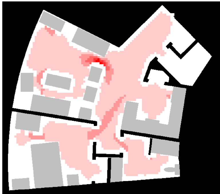
Figure 3.2: Coverage utility heat-map of a person walking in the Independent Living Suit (ILS).
