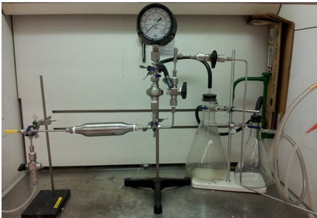
Figure 3.1: 1st Prototype Reactor Design for the oxidation of MFT samples
