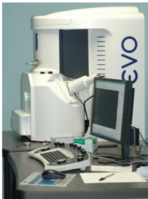
Figure 3.9: Scanning Electron Microscope used for surface analysis of sediment after WAO/WAPO (Source: Earth and Atmosphere Science; University of Alberta, 2014 )
