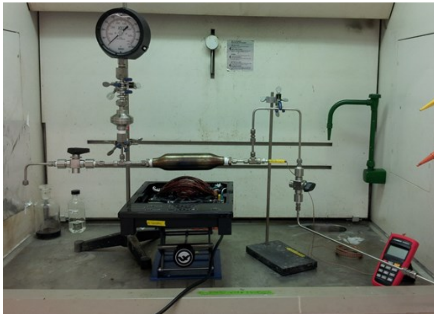
Figure 3.3: 2nd Prototype Reactor Design for the oxidation of MFT samples
