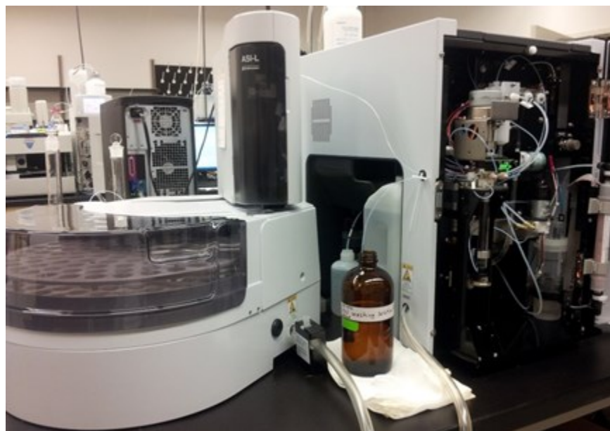
Figure 3.5: TOC-LCPH/CPN Analyzer equipped with ASI-L Auto-sampler used for TOC/NPOC and TIC measurement
