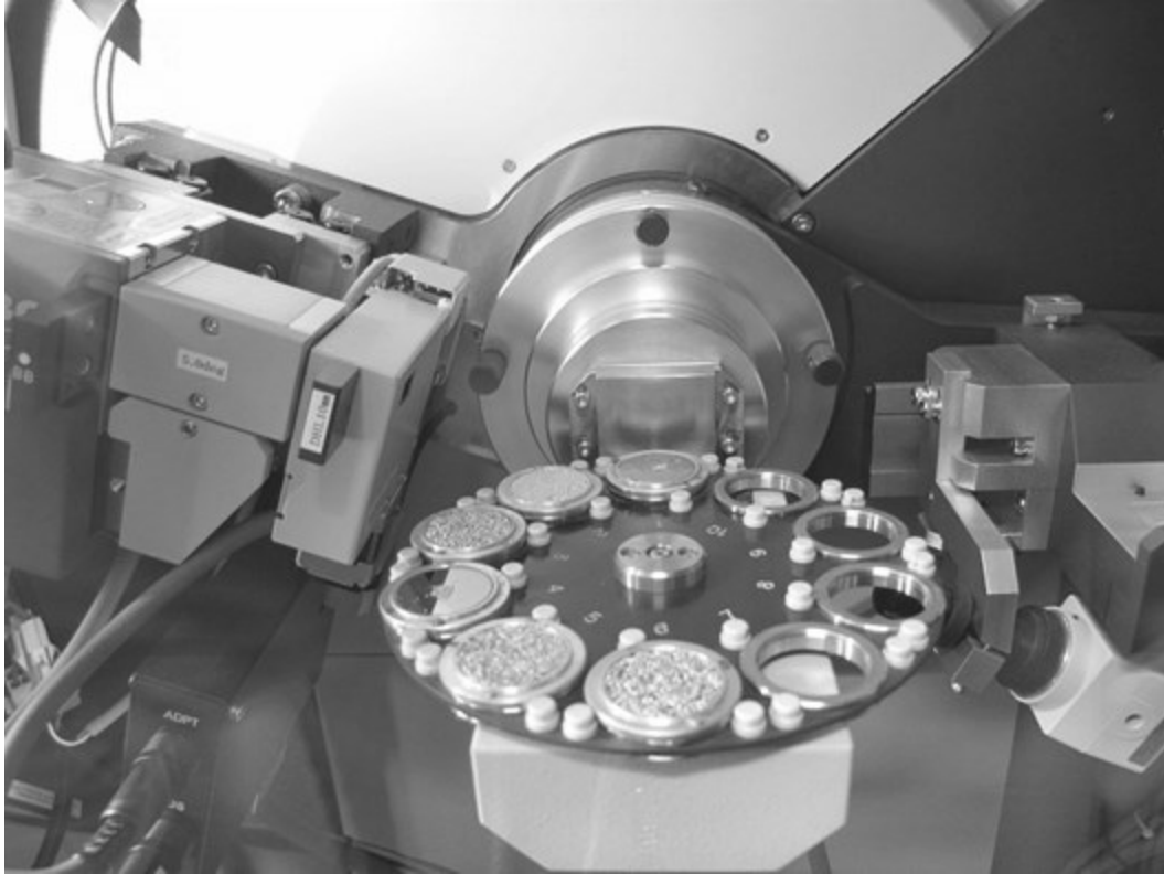
Figure 3.8: Rigaku Ultima IV unit's 10-position sample chamber during sample analysis
