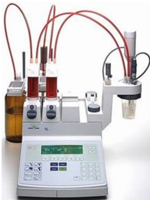
Figure 3.6: Mettler Toledo DL53 autotitrator used for alkalinity measurements
