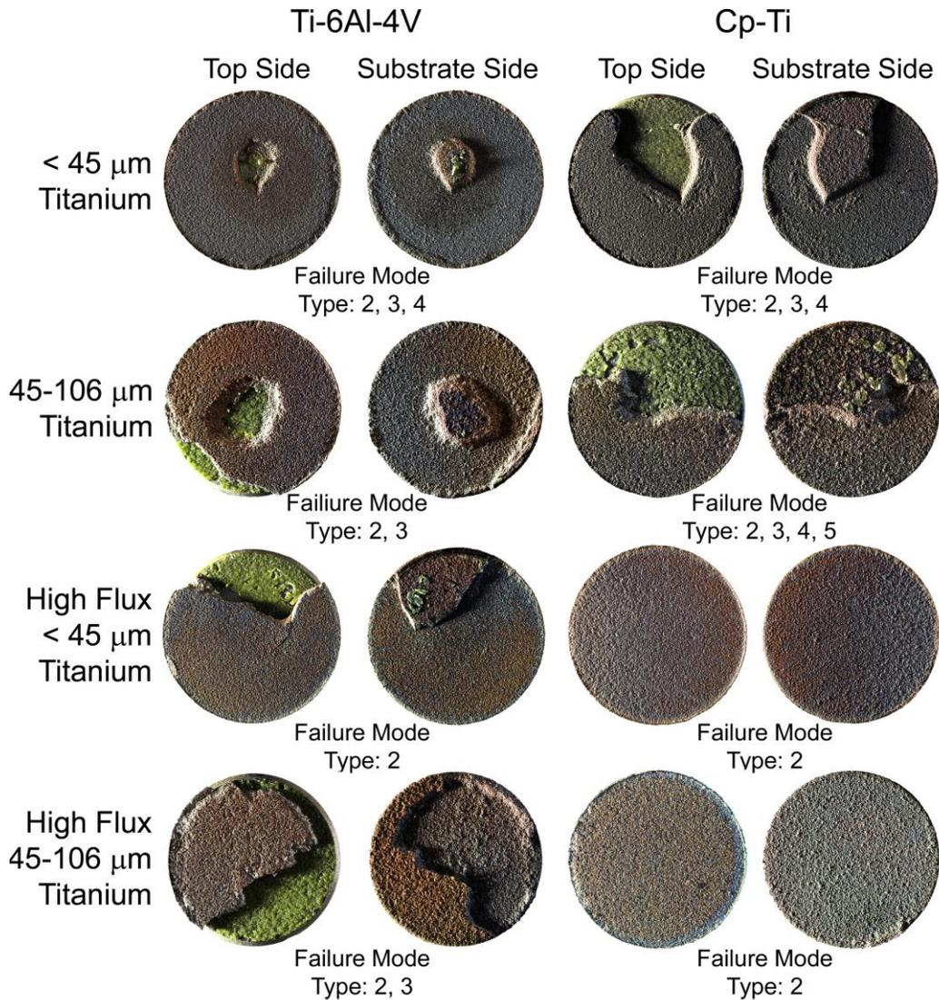
**Figure 5-36.** Representative fractographs of failed control coatings after ASTM Standard C633 tensile adhesion testing taken by macrophotography. Failure mode type legend: 1. Coating-substrate adhesive failure, 2. Coating cohesive failure, 3. Coating-epoxy adhesive failure, 4. Epoxy cohesive failure, and 5. Epoxy-stub adhesive failure.
