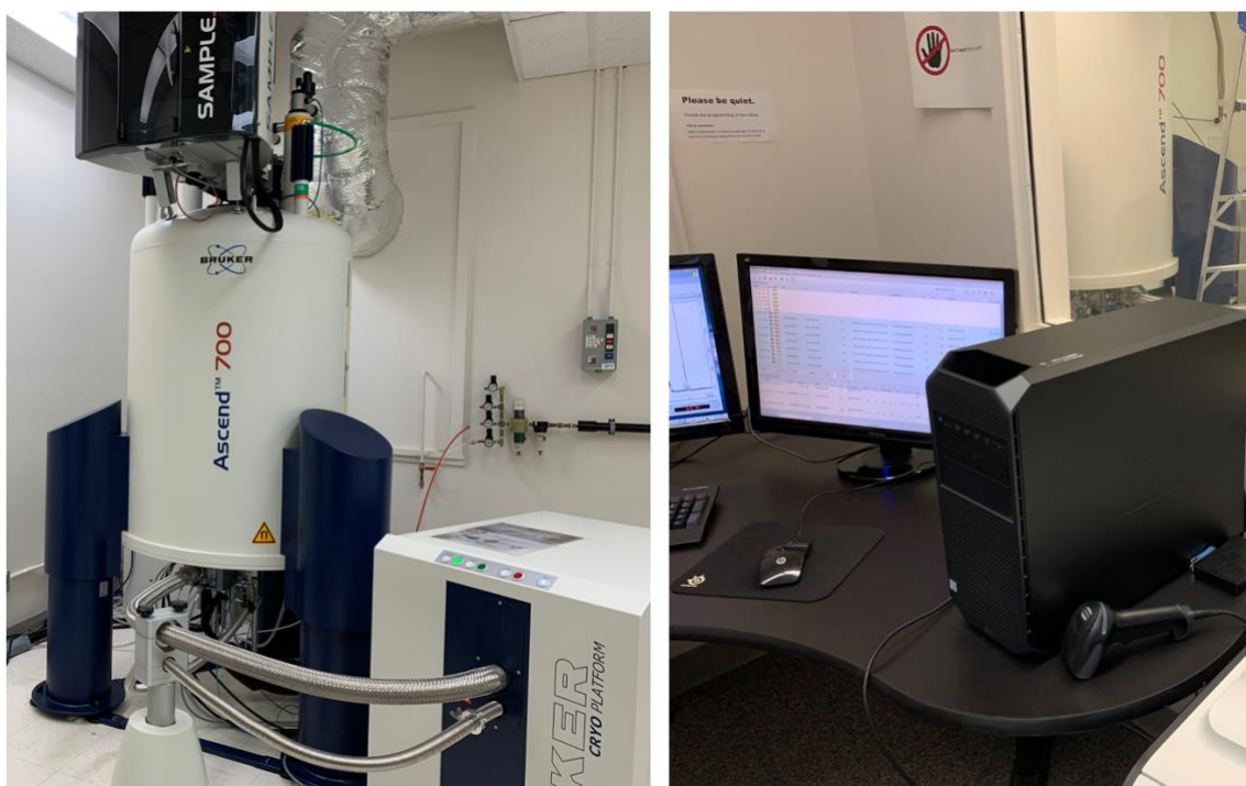
Figure 1.1: An NMR spectrometer (left side) and its computer terminal (right side)
