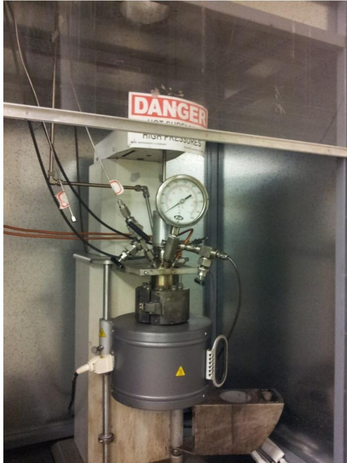
**Figure 3.4 Hydrothermal dewatering autoclave**
