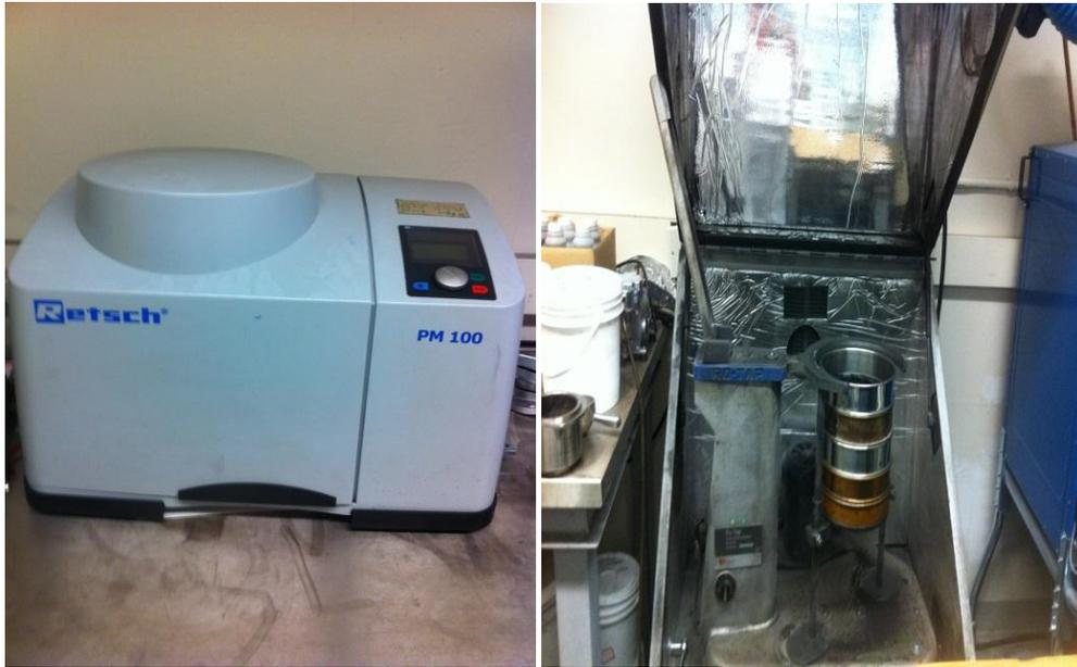
**Figure 3.1 Grinder and sieves**
