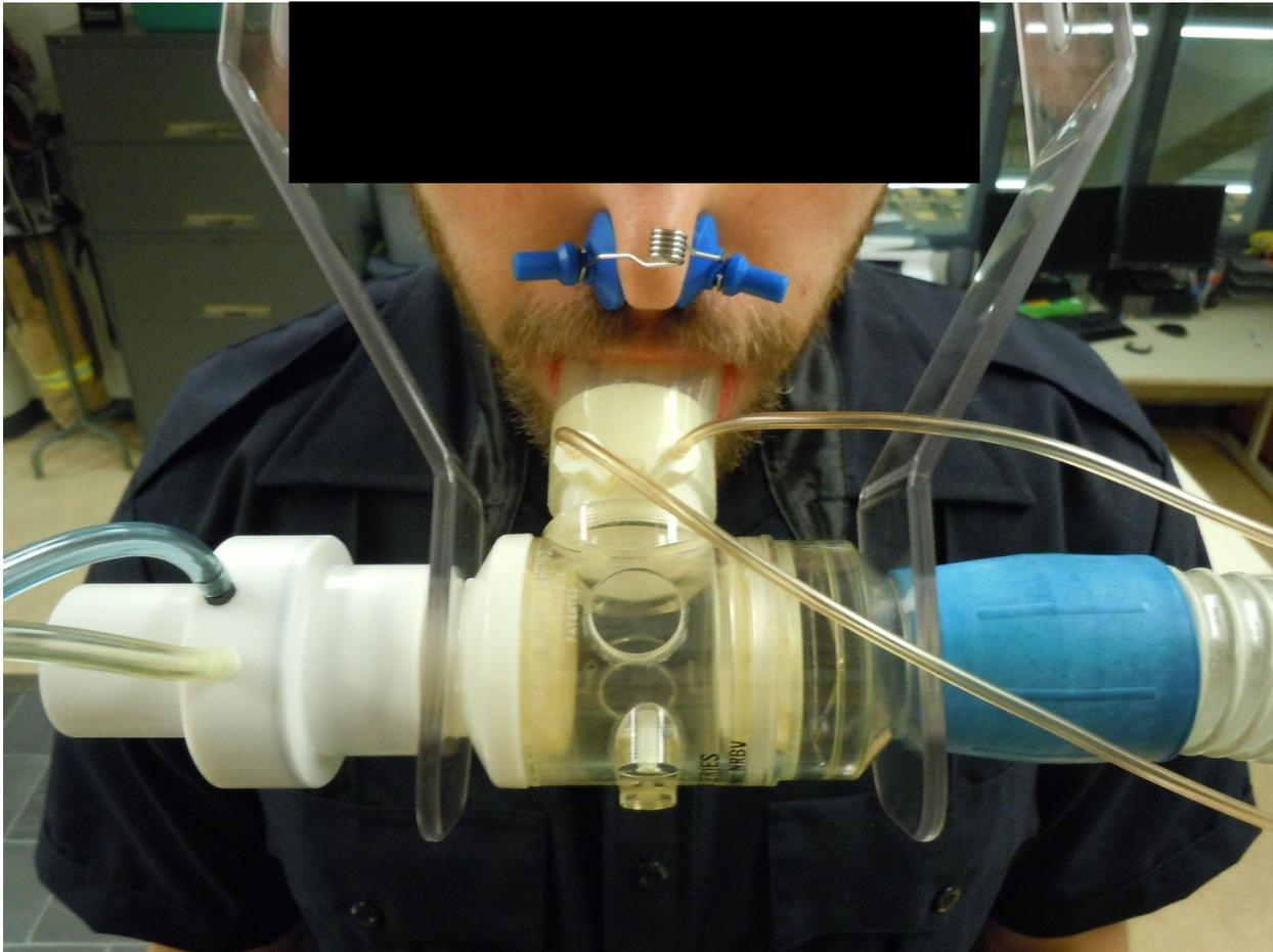
Plate A-1. The two-way, non-rebreathing valve (Hans Rudolph, Kansas City, MO, USA) with: inspiratory pneumotach (left), ports for ET $\text{CO}_2$  and mouth pressure (top), and expired gas collection (right).
