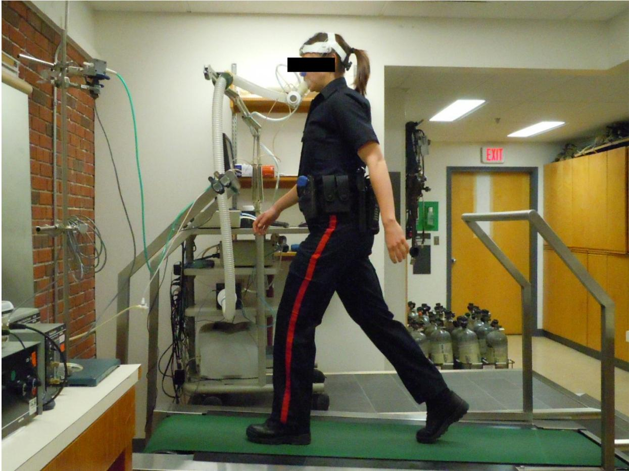
Plate A-6. The complete experimental apparatus with a subject walking on the treadmill in the PDE (police duty ensemble) condition.
