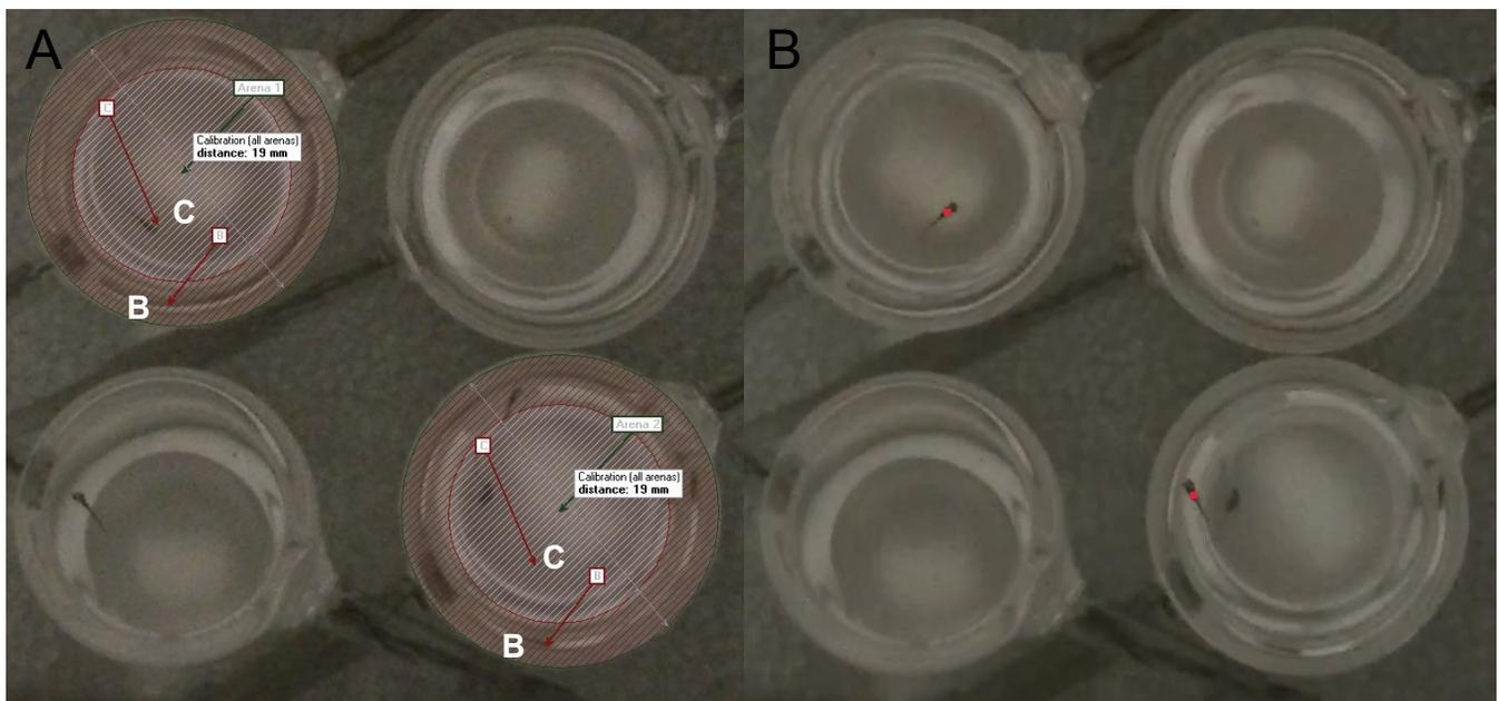
**Figure 2.8.** Sample image of EthoVision XT arena set up and tracking. A) Arena settings. White B and C letters indicate border and centre zones respectively. Chamber image is calibrated to real life diameter of 19mm. B) Screenshot of movement tracking in progress. Red marker identifies centre point of the fish.
