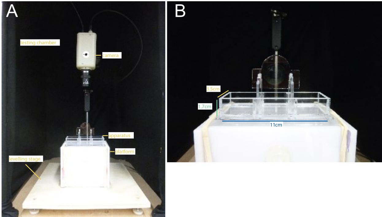
**Figure 2.1.** Avoidance-attraction apparatus experimental setup. A) Entire system within curtained enclosure. B) Close up and dimensions of apparatus.
