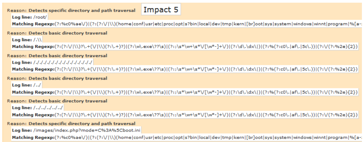
Figure-8: Dshield logs as a result from the automated Nikto scan for Remote file inclusion
