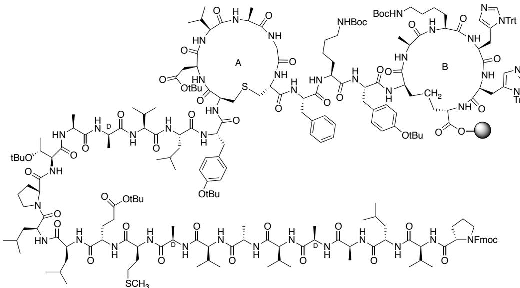
Following protocol D, residues 37-3 (**177**) of B-DAP lactocin S were synthesized. Briefly, the amino acids corresponding to residues 21-3 were introduced to **177a** via Fmoc-SPPS and then a small sample was cleaved from the resin and analyzed by MALDI-TOF MS: Calculated for  $C_{182}H_{270}N_{41}O_{45}S_2$  3815.5, found 3815.8  $(M+H)^+$ .
