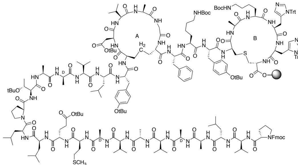
Following protocol D, residues 37-3 (**173**) of A-DAP lactocin S were synthesized. Briefly, the amino acids corresponding to residues 21-3 were introduced to **172** via Fmoc-SPPS and then a small sample was cleaved from the resin and analyzed by MALDI-TOF MS: Calculated for  $C_{182}H_{270}N_{41}O_{45}S_2$  3815.5, found 3816.0  $(M+H)^+$ .
