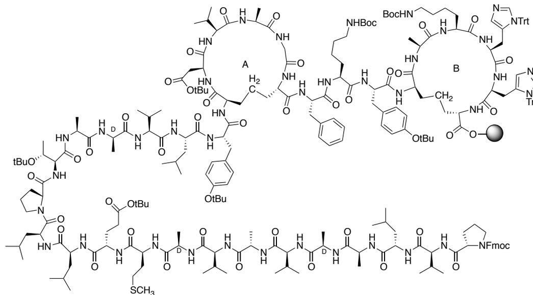
Following protocol D, residues 37-3 (**178**) of DAP lactocin S were synthesized. Briefly, the amino acids corresponding to residues 21-3 were introduced to **178a** via Fmoc-SPPS and then a small sample was cleaved from the resin and analyzed by MALDI-TOF MS: Calculated for  $C_{183}H_{272}N_{41}O_{45}S$  3797.4, found 3799.0  $(M+H)^+$ .
