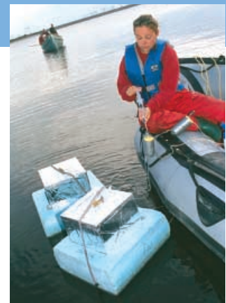
Floating chambers for measuring GHGs
