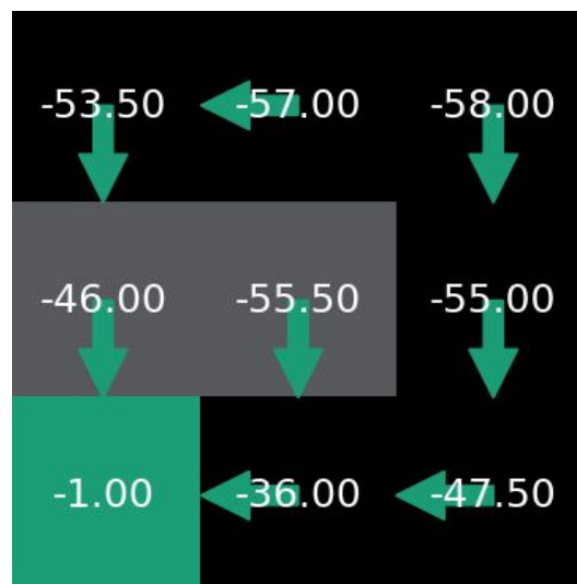
Figure C.1: A simple ElectricProcMaze instance showing the greedy policy (green arrows) and associated action values under the uniform random policy. The values printed on each cell are the action values associated with moving into that cell from any other cell which works in this case since the reward is determined by the cell being entered regardless of the origin. The action values were computed by explicitly solving the Bellman equation with a uniform random behaviour policy. The reward for entering a wall cell is -7 in this case which is one less than the return achievable by following an optimal policy from the furthest cell to the goal. Hence the optimal policy will never enter a wall cell, but the greedy policy with respect to the action values of the uniform random policy does.
