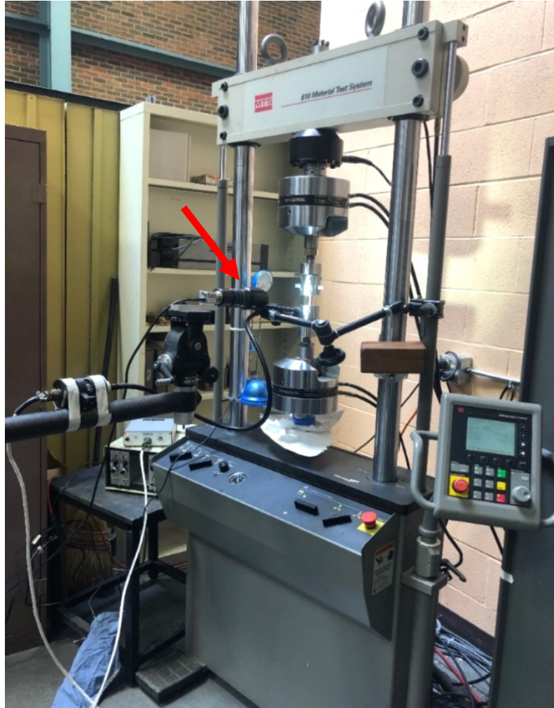
Figure 15: Image of the MTS machine that was used to conduct the tensile tests. The arrow shows the Promon U750 high speed camera that was used to capture the deformation video to be used as an input to DIC.
