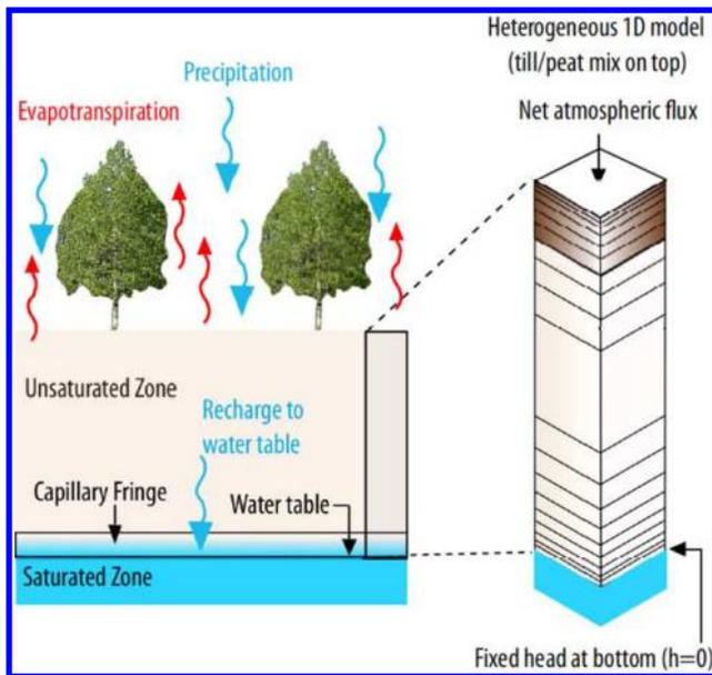
Fig. 2. Virtual experiment set up showing the boundary conditions and variable discretization used.
