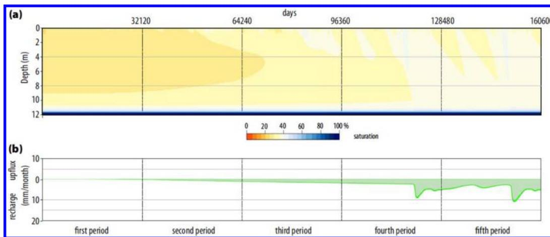
**Fig. 7.** Complete simulation for the 12-m tailings sand profile showing: (a) daily soil water and (b) monthly fluxes at the water table aggregated from daily values. Each period covers the 88 yr or 32 120 d with data from Fort McMurray. Fluxes at the water table stabilize toward the last third of the fourth period, thus requiring more than 308 yr of spin up time.
