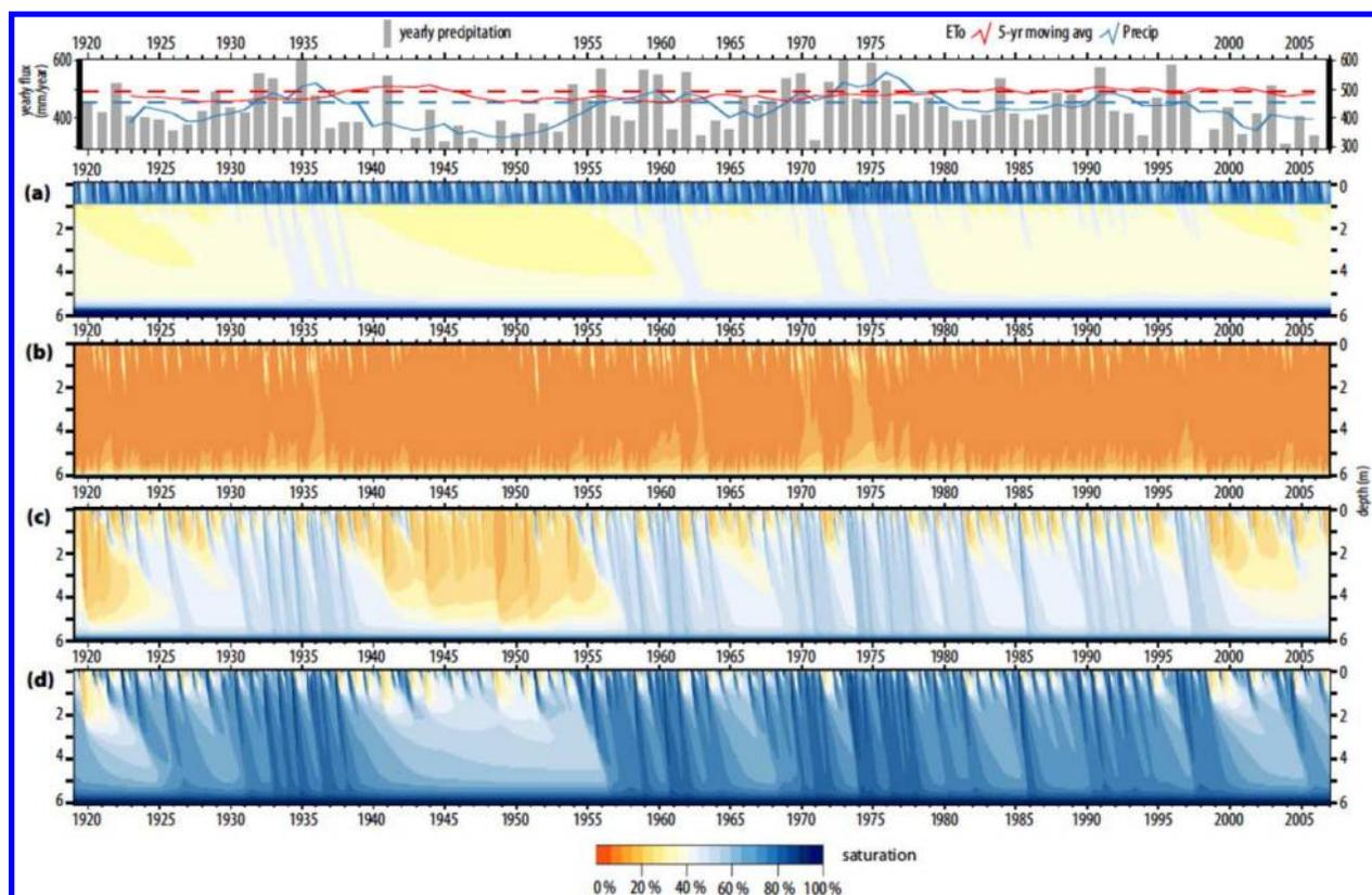
**Fig. 10.** Daily soil water dynamics for a water table fixed at a depth of 6 m for different materials (a) reclamation scenario with 1 m of till and peat mix on top, (b) sand, (c) sandy loam and (d) loam. The top plot shows the variability of the climate conditions for the simulated period (1919–2006) along with their respective normals (1971–2000).
