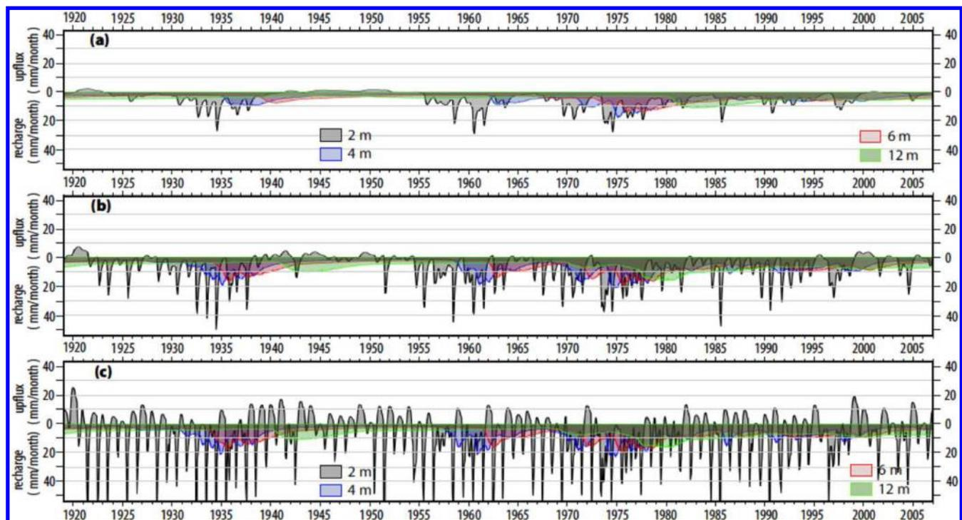
Fig. 11. Monthly fluxes at the water table for different depths (2, 4, 6 and 12 m) for three different depths of capping material on top of tailing sands (a) 0 m, (b) 0.5 m and (c) 1.0 m. These monthly fluxes were aggregated from daily data to improve their visualization.
