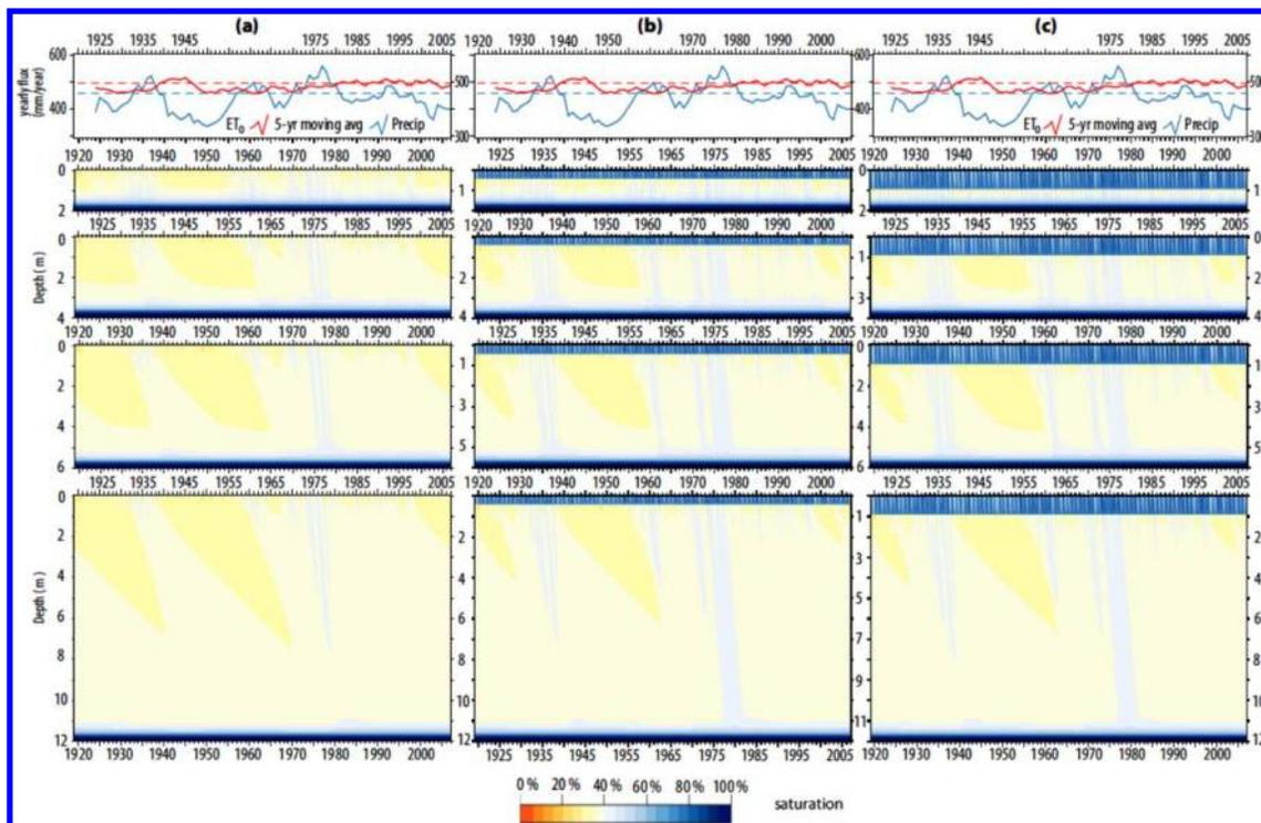
Fig. 9. Daily soil water dynamics for different depths of capping material used on top of tailings sand: (a) 0 m, (b) 0.5 m and (c) 1.0 m considering different water table depths commonly found on the boreal plains (2, 4, 6 and 12 m). The top plot shows the variability of the climatological conditions for the simulated period (1919–2006).
