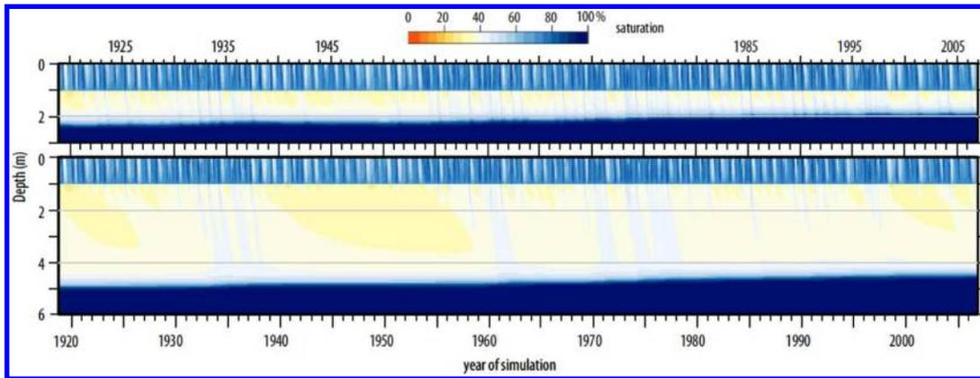
Fig. 8. Water table fluctuation for different initial water table depths; water table rises slowly, even for the shallowest case shown.
