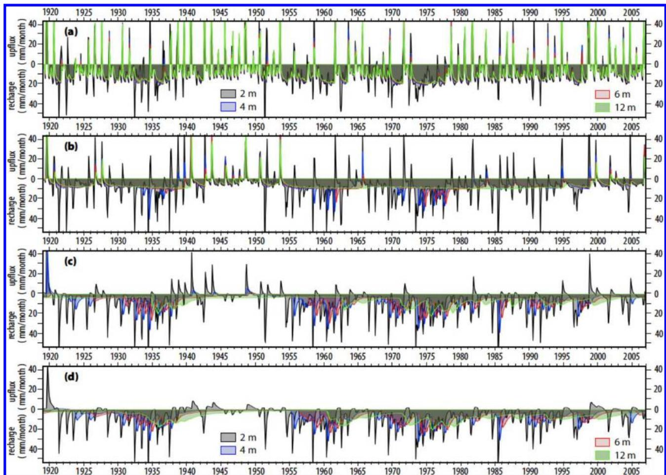
**Fig. 12.** Monthly fluxes at the water table for different depths (2, 4, 6 and 12 m) for four different soil textures found on the Boreal Plain: (a) sand, (b) loamy sand, (c) sandy loam, (d) loam. These monthly fluxes were aggregated from daily data to improve their visualization.
