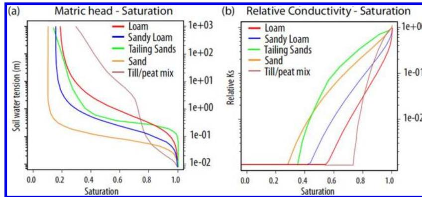
**Fig. 3.** Saturation curves for tailing sands, sand, loamy sand, sandy loam and loam; (a) saturation matric head and (b) saturation relative  $K_s$ . Curves are based on tabular values determined from the van-Genuchten parameters of Carsel and Parrish (1988) for natural materials. For tailings sand, these curves were developed from the values provided in Syncrude (2007), while those for the peat and till mix were taken from Shurniak and Barbour (2002).
