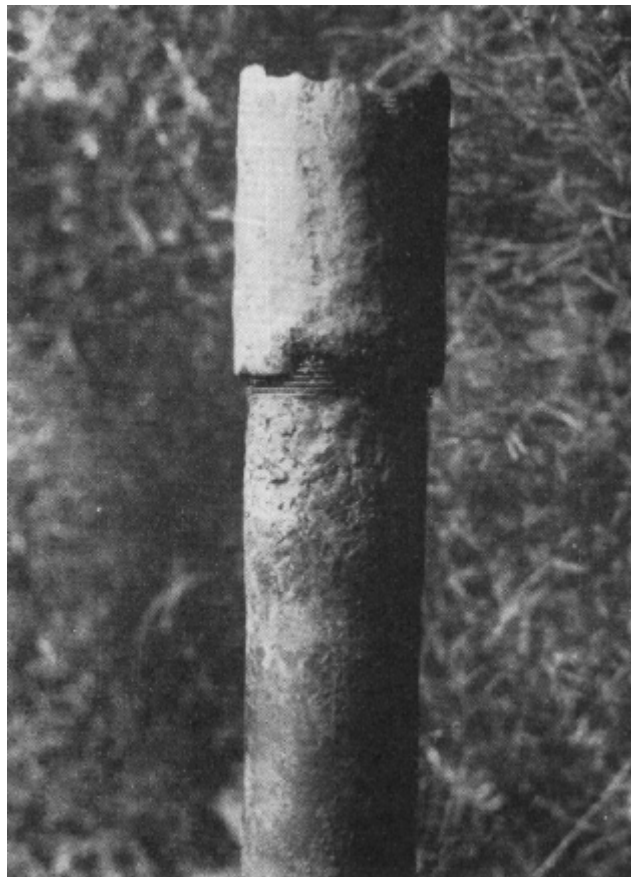
Figure 2.2: Hydrogen sulfide corrosion attack of oil well tubing after 24 months of service [13].
