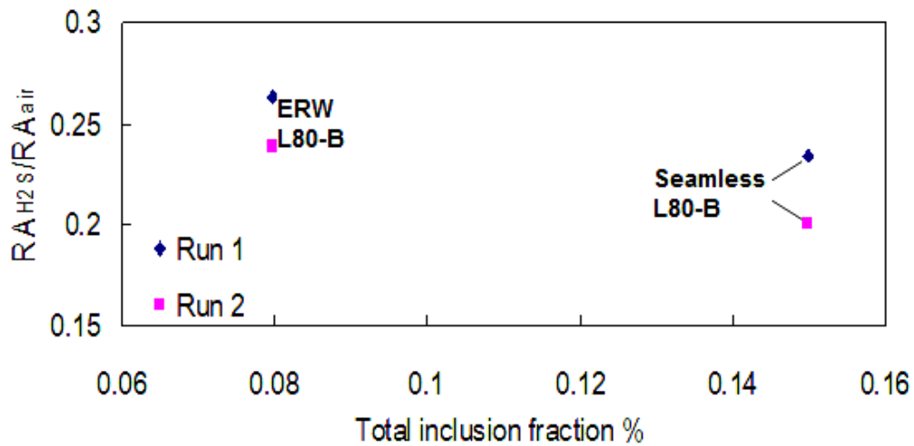
Figure 4.40: Total inclusions fraction % vs. RAR for Ti-B steels.
