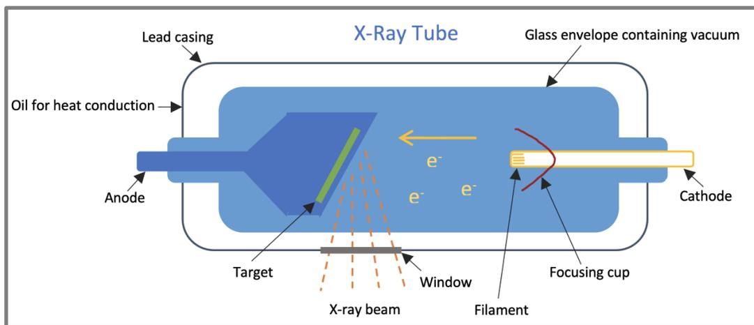
Figure 2.2 Simple schematic of X-ray tube.
