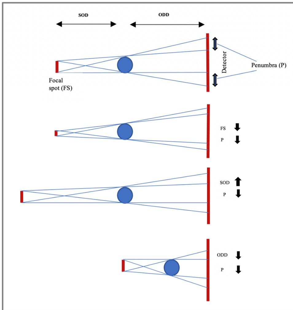
*Figure 2.3 Effect of Focal Spot (FS) size. Source to Object Distance (SOD), Object to Detector Distance (ODD), penumbra (P). Small FS, larger SOD and smaller ODD all reduce the penumbra width hence increase image sharpness.*
