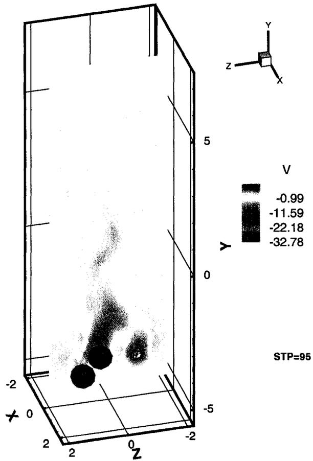
Figure 9.49: Three spheres in a vertical arrangement. Numerical results:  $t=95dt$ . Contour at  $X=0.12$  (dimensionless).
