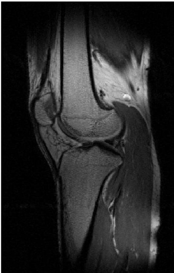
Figure 5-4 (left): A proton image (fast spin echo, TE = 15 ms, TR = 4 s) of a knee using the double tuned concentric coil. Variations in signal strength are seen within similar tissues, indicating imperfect homogeneity in the coil.
