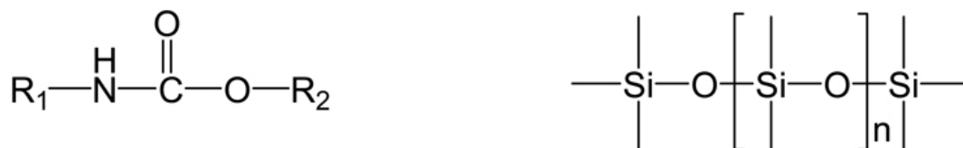
Figure 2-1. Chemical structures of “non-biodegradable” polymers used for drug delivery. The first structure from the left is urethane links and the second structure is polydimethylsiloxane.
