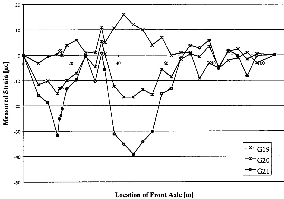
Figure B14: Static Load Test, August '98 for Girder 2 in Negative Moment Region
