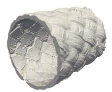
Figure 3-3: Three dimensional braid geometry recreated from  $\mu$ CT images
