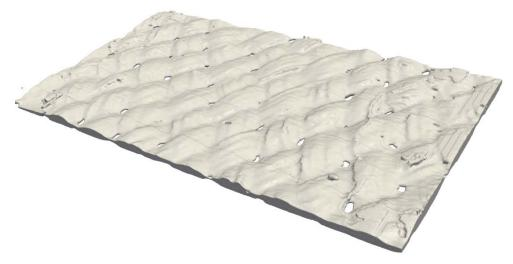
Figure 3-9: Unwrapped 3D braid geometry created using the unwrapped two dimensional braid images
