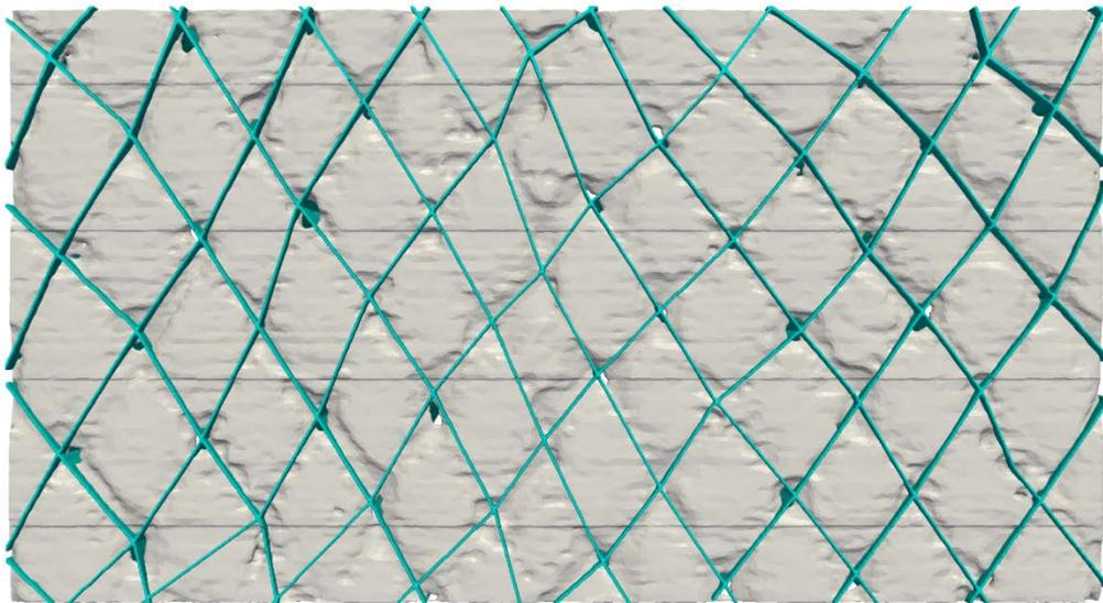
Figure 3-10: Segmentation of braid yarns using the 3D braid geometry created using SimpleWare
