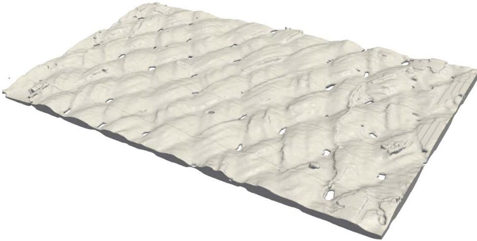
Figure 3-9: Unwrapped 3D braid geometry created using the unwrapped two dimensional braid images
