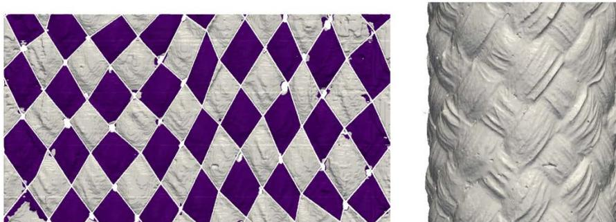
Figure 3-12: Unwrapping of original cylindrical  $\mu$ CT scans. Left: original tubular braid geometry. Right: unwrapped braid geometry with individual yarns identified.
