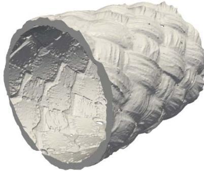
Figure 3-3: Three dimensional braid geometry recreated from  $\mu$ CT images
