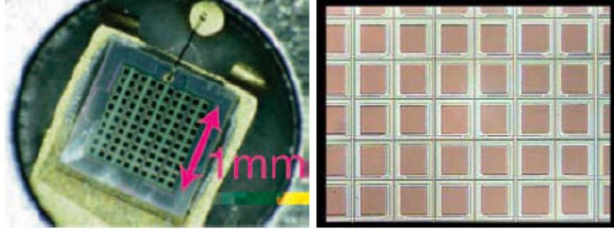
Figure 3.19: Picture of a 100 pixel MPPC and a close up view showing each pixel of the device [2]. The pixel size is  $100 \times 100 \text{ }\mu\text{m}$  each.
