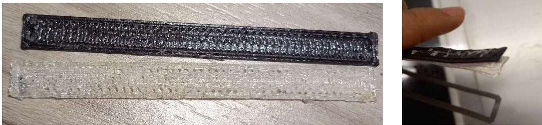
Figure 4.4. Delamination between layers in specimen, layers completely separated showing a clean surface (left), as printed sample (right)
