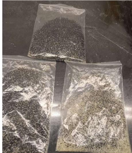
Figure 4.5. Different percentages of carbon fiber and SMP.
