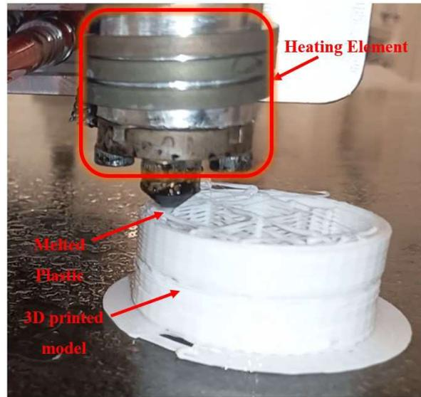
Figure 2.2. Big format 3D printer model 300Workbench from 3D Platform printing a cylinder.
