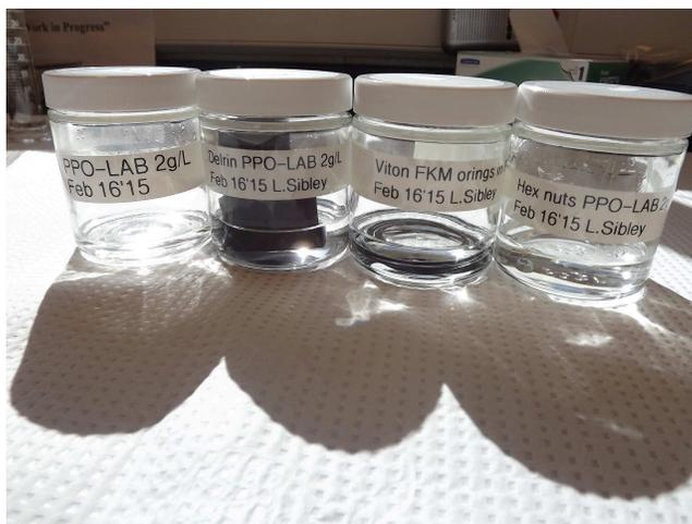
Figure 4.19: Samples of the Delrin<sup>®</sup>, Viton<sup>®</sup> o-rings and stainless steel nylon-insert lock nuts soaked in LS for seven months. SNOLAB technicians performed UV/VIS scans at various times to check for changes in the LS absorbance, which would indicate material incompatibility.
