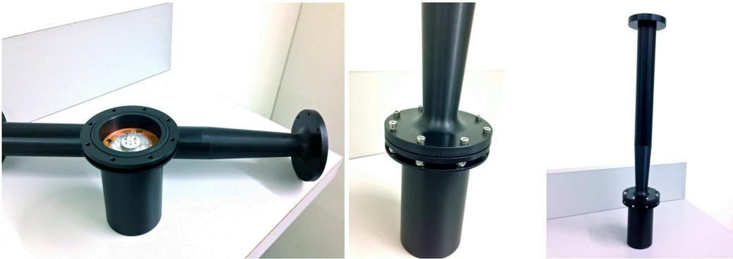
Figure 4.17: The Delrin<sup>®</sup> encapsulation consists of a container with 2 mm thick walls that houses the copper encapsulation (left). Eight screws connect this container to a stem at a flange (middle), which compresses an internal o-ring to provide a leak-tight seal. When connected (right), the Delrin<sup>®</sup> layer is nearly 398 mm in height. This does not include the source connector that will attach to the top of the stem.
