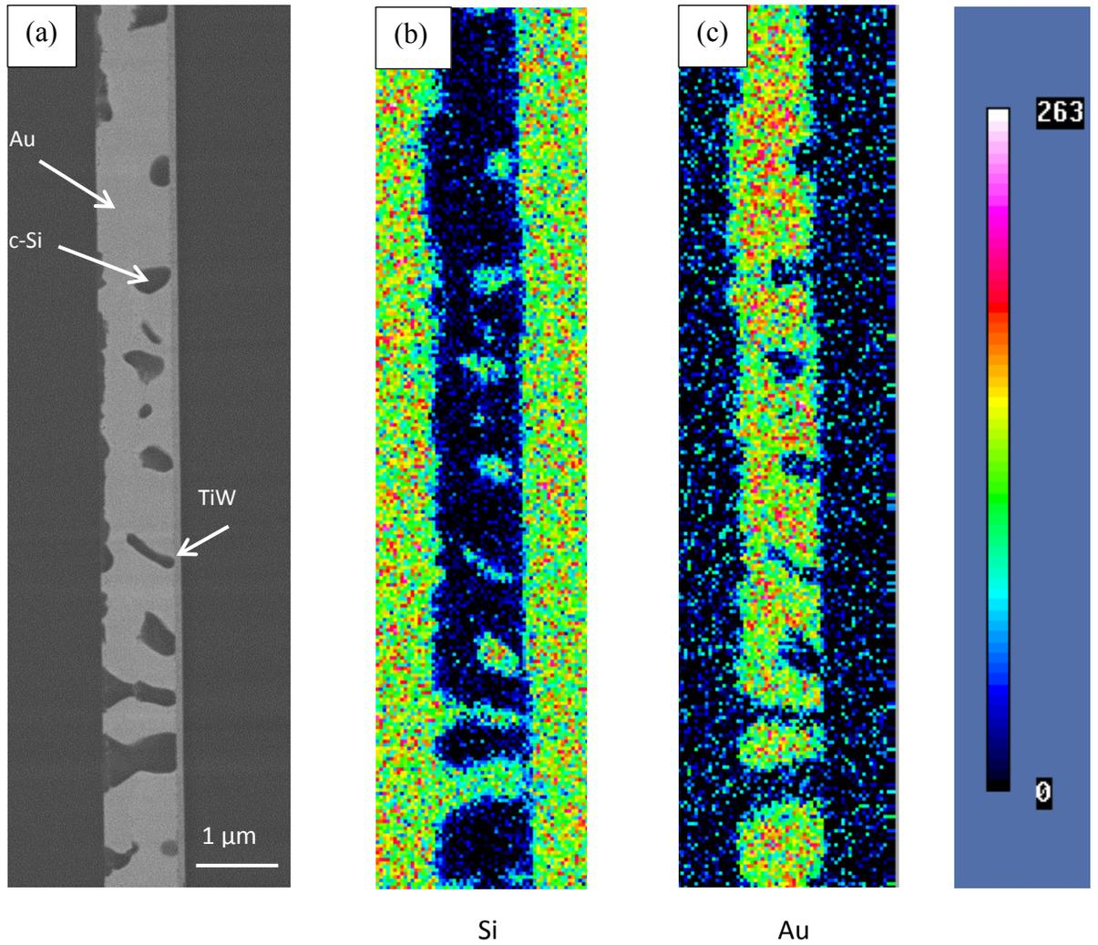
Figure 6.4. AES maps taken from the (a) SE SEM cross section image. (b) Si map and (c) Au map of an a-Si eutectic bonded sample preheated to 350°C for 20 min and bonded at 400°C for 15 min.
