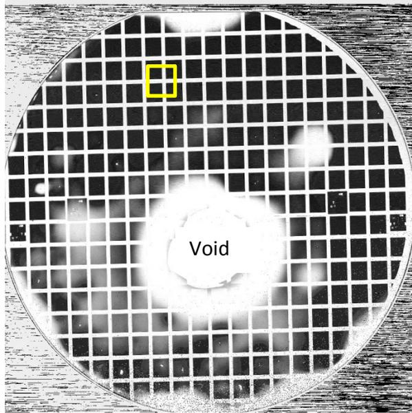
Figure 6.14. SAM image for c-Si solid state pair bonded at 350°C for 20 min at a pressure of 0.12 MPa.
