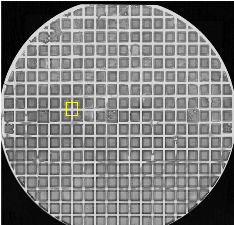
Figure 6.8. SAM image for full wafer eutectic bonding of c-Si with SC1 and HF cleaning prior to bonding.
