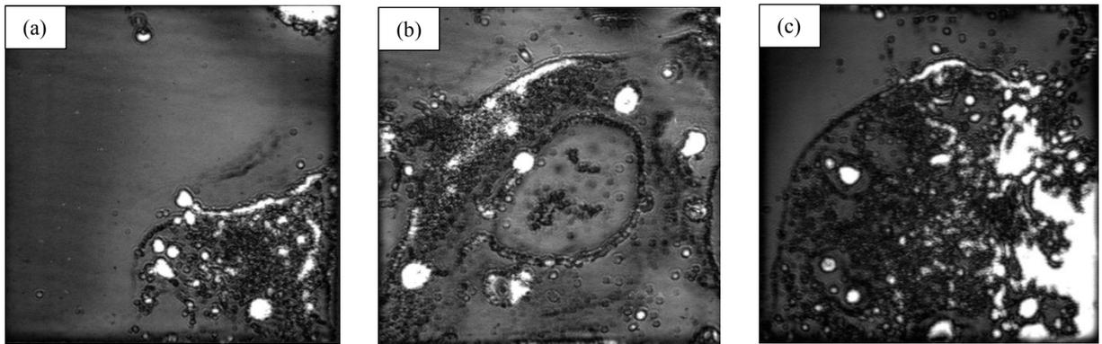
Figure 5.27. SAM images of three a-Si/Au samples that were solid-state bonded at 350°C for 10 min. The sample location on the chuck was position 1 in Figure 5.11.
