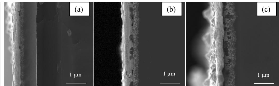
Figure 4.4. SEM SE images of cleaved cross sections for Au/a-Si diffusion couples annealed at
