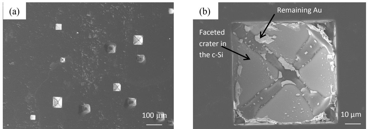
Figure 5.23. Plan view SEM SE images from detached pieces bonded at 425°C for 30 min (sample 3): (a) low magnification and (b) high magnification.
