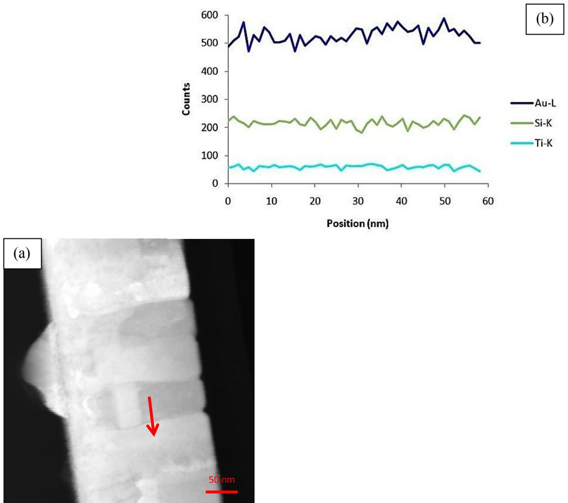
Figure 4.18. (a) STEM HAADF image of a cross section specimen from the Au/Ti/c-Si sample annealed at 350°C for 30 min. (b) X-ray line scan across a grain boundary (indicated by the arrow in (a)).
