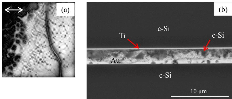
Figure 5.3. Cross section BSE image (b) of the region indicated by the arrow in SAM image (a) for an a-Si sample bonded at 400°C for 30 min (sample 2).
