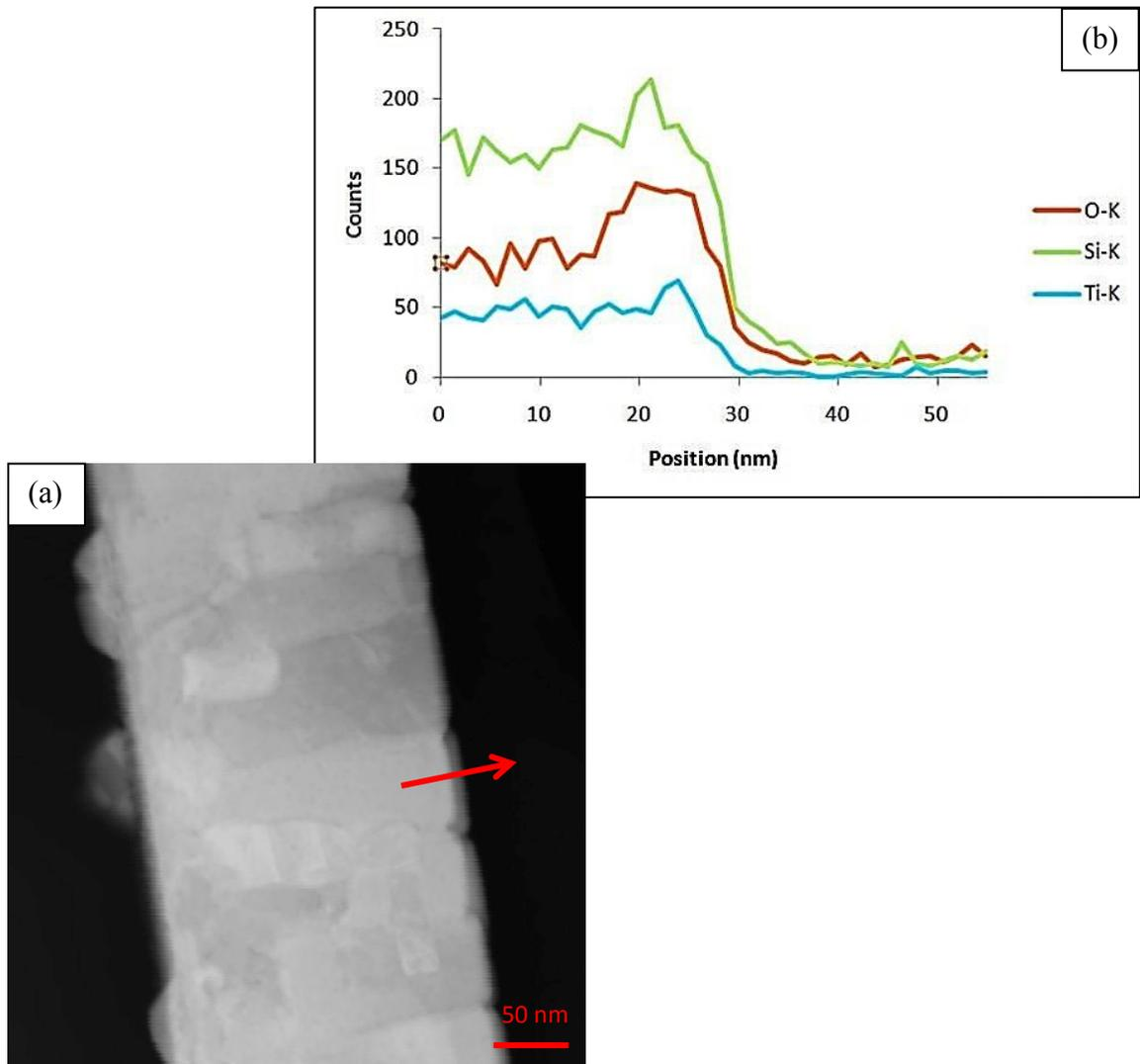
Figure 4.17. (a) STEM HAADF image from a cross section of the Au/Ti/c-Si sample annealed at 350°C for 30 min. (b) X-ray line scan across the oxide layer in (a) (indicated by the arrow).
