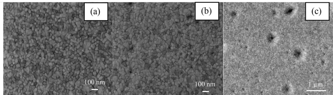
Figure 4.12. SE SEM images of hole formation on the Au surface at (a) 250°C, (b) 300°C and (c) 350°C for samples annealed for 30 min.
