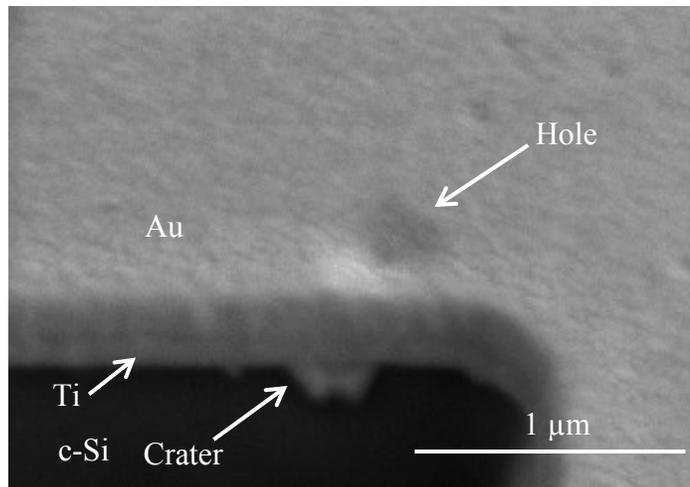
Figure 4.13. SEM SE image of crater/void formation during annealing of a Au/Ti/c-Si couple at 350°C for 30 min.
