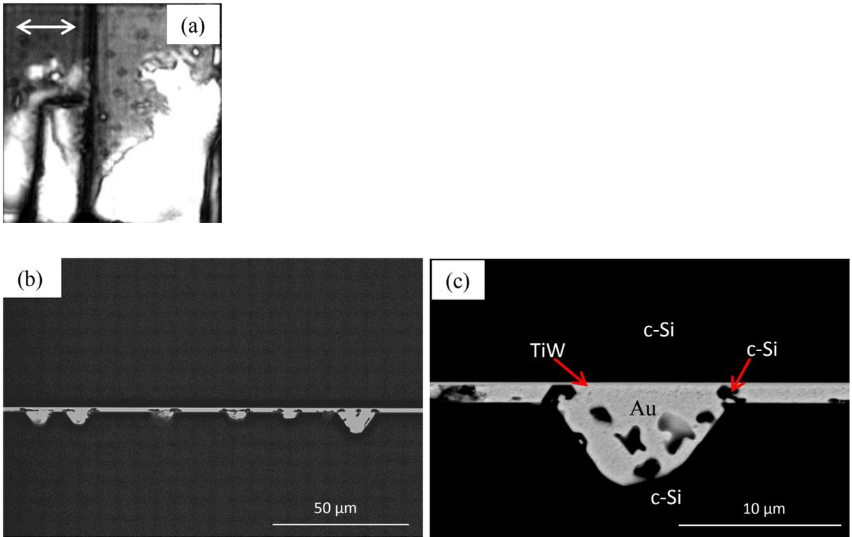
Figure 5.22. Cross section BSE SEM images (25 kV) from the interface of Au/c-Si sample 3 bonded at 425°C for 30 min; taken from the region indicated by the arrow in the SAM image (a): (b) low magnification and (c) high magnification.
