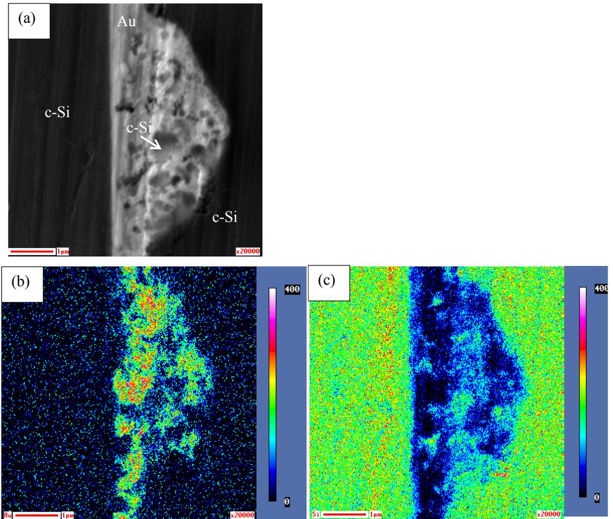
Figure 5.20. (a) SEM SE cross section image of the crater area from the c-Si sample bonded at 400°C for 30 min. AES maps for Au (b) and Si (c) (sample 1).
