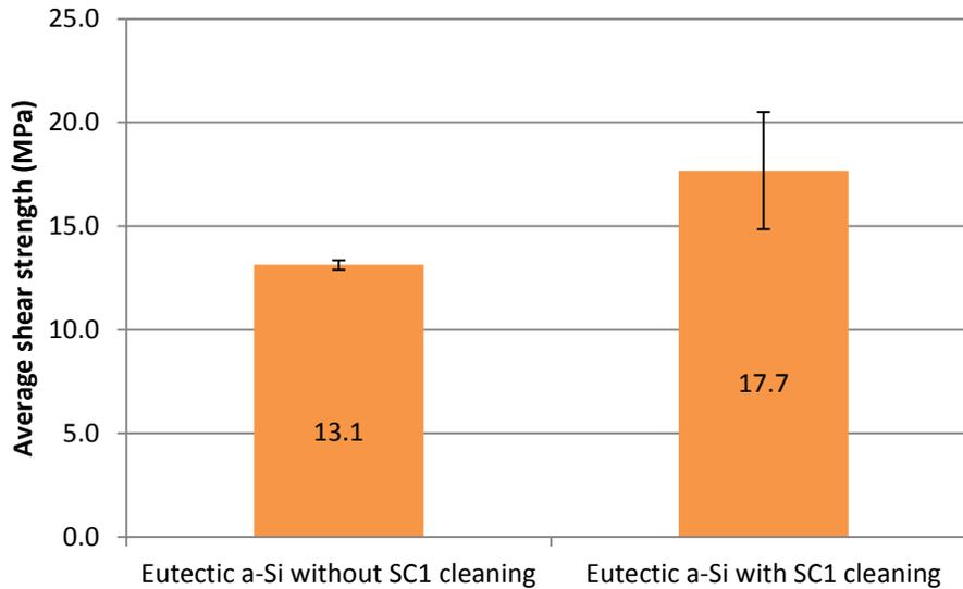
Figure 6.17. Average shear strength comparison of a-Si eutectic bonded samples with and without SC1 cleaning prior to bonding.
