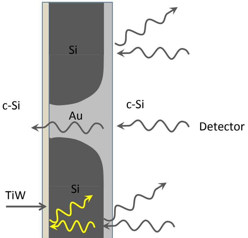
Figure 5.14. Schematic image of bonded interface and sound wave reflection from the Au/c-Si interfaces. The reflections are detected by the detector and therefore areas with more reflections appear bright in SAM images compared with areas with fewer or no reflections.
