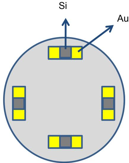
Figure 3.2. Four sample configuration used on the chuck in order to improve pressure uniformity.
