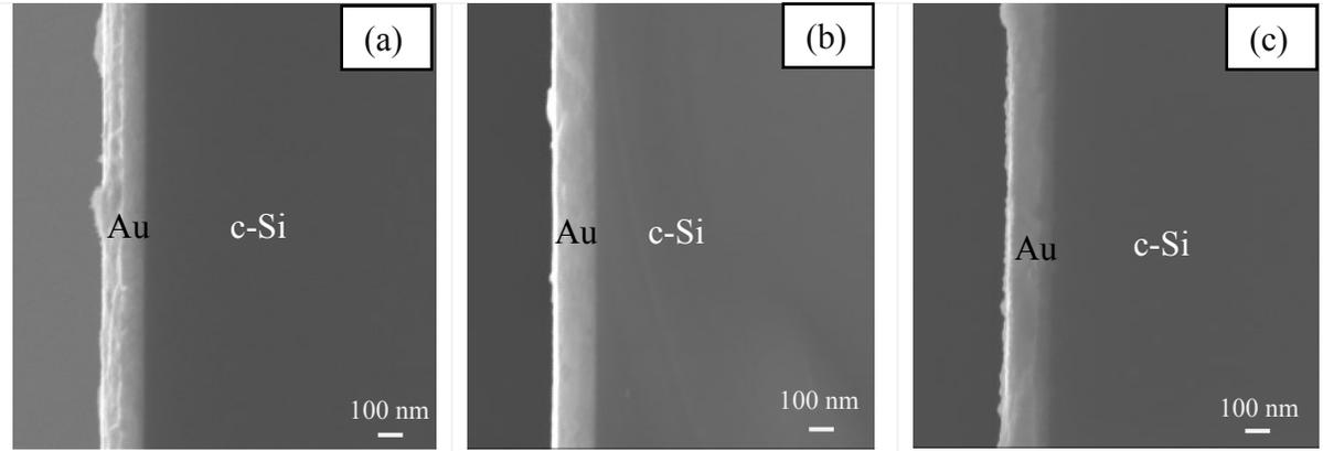
Figure 4.10. SEM SE images of cleaved cross sections for Au/c-Si diffusion couples annealed at 300°C for (a) 10 min, (b) 20 min and (c) 30 min.
