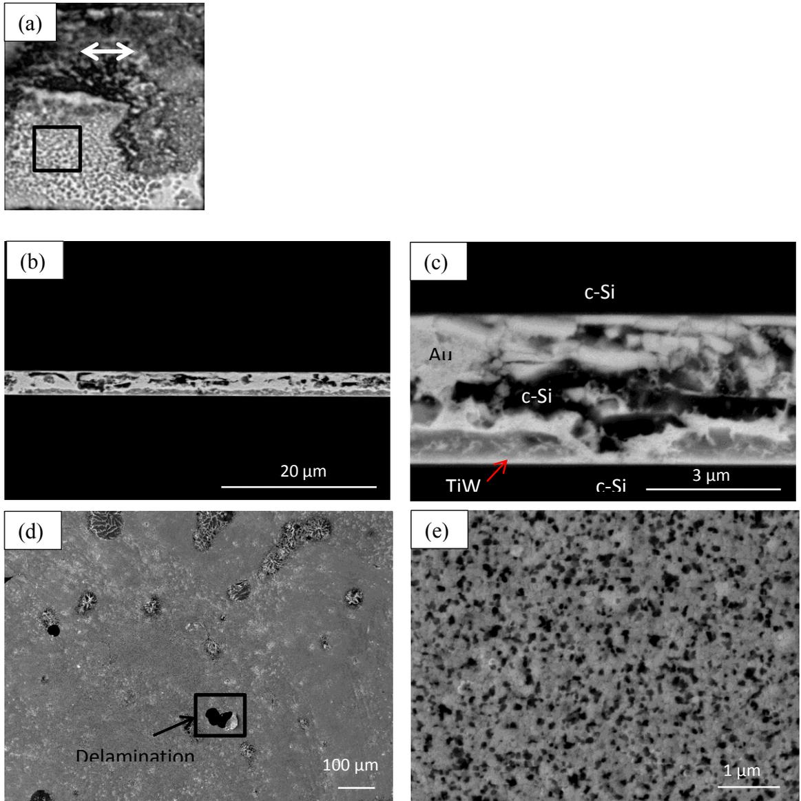
Figure 5.5. Images taken from the Au side of sample 3 (a-Si bonded at 425°C). (a) SAM image, (b) low magnification and (c) high magnification SEM BSE cross section images from the region indicated by the arrow in (a). (d) Low magnification and (e) high magnification SE plan view images of the detached pieces from the black square shown in (a).
