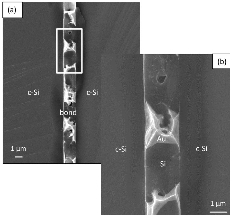
Figure 5.29. SEM SE cross-section images from region indicated by the yellow rectangle in Figure 5.28(b): (a) Low magnification image and (b) higher magnification image of region indicated in (a).
