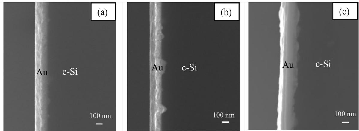
Figure 4.11. SEM SE images of cleaved cross sections for Au/c-Si diffusion couples annealed at 350°C for (a) 10 min, (b) 20 min and (c) 30 min.
