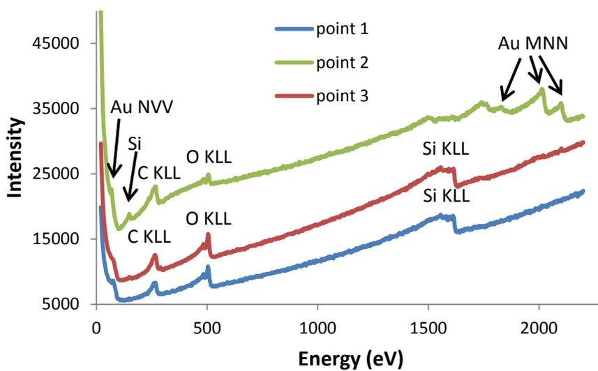
Figure 5.19. AES spectra obtained from points 1, 2 and 3 in Figure 5.18.
