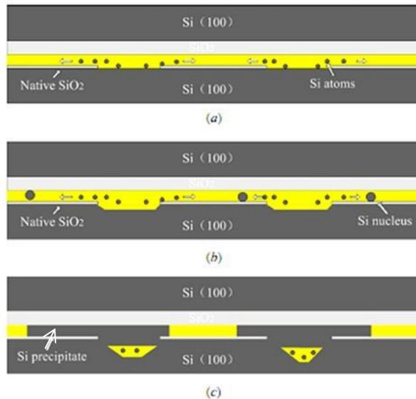
Figure 2.8. Schematic illustration showing the formation mechanism at the Au/Si bond interface. a) Si dissolution and diffusion; b) formation of Si nuclei; c) growth of Si precipitates and refilling of Au [48].
