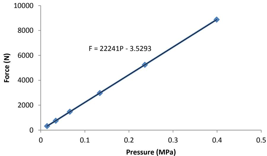
Figure 3.3. Force versus pressure plot for the bonder.
