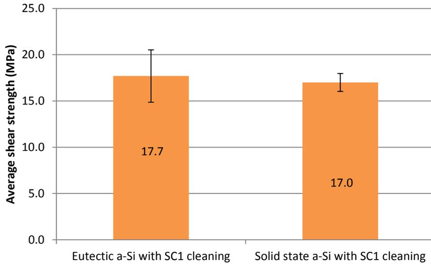
Figure 6.18. Average shear strength comparison of a-Si eutectic bonded samples with solid-state bonded samples.
