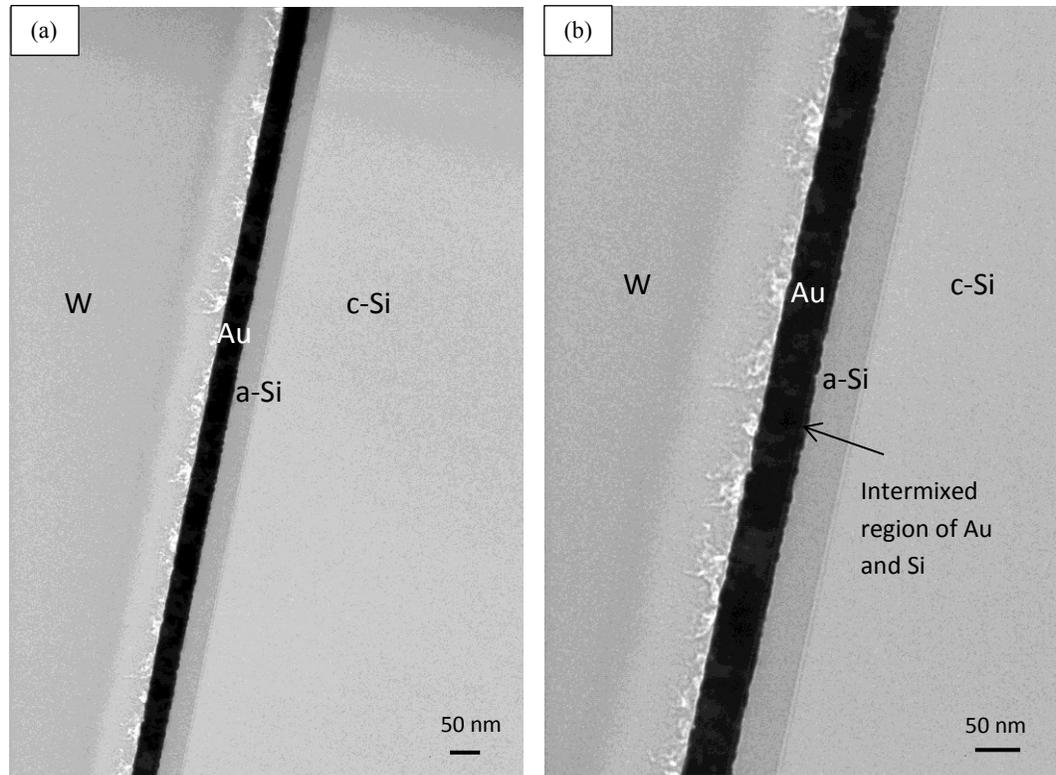
Figure 7.1. BF TEM cross section images of FIB polished Au/a-Si/c-Si sample before annealing. (a) Low magnification and (b) higher magnification images.
