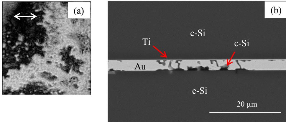
Figure 5.2. Cross section BSE image (b) of the region indicated by the arrow in SAM image (a) for an a-Si sample bonded at 400°C for 30 min (sample 1).
