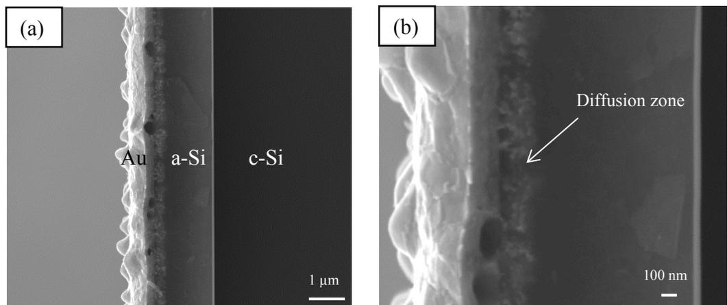
Figure 4.1. SEM SE images of a cleaved cross section for as-deposited Au/a-Si/c-Si diffusion couple: (a) low magnification image and (b) higher magnification image. The sample was stored for 2 weeks at room temperature prior to imaging.
