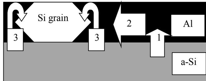
Figure 4.7. Schematic diagram of the diffusion and interface processes involved in the grain growth [79].
