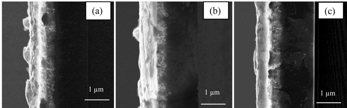
Figure 4.3. SEM SE images of cleaved cross sections for Au/a-Si diffusion couples annealed at 250°C for (a) 10 min, (b) 20 min and (c) 30 min.
