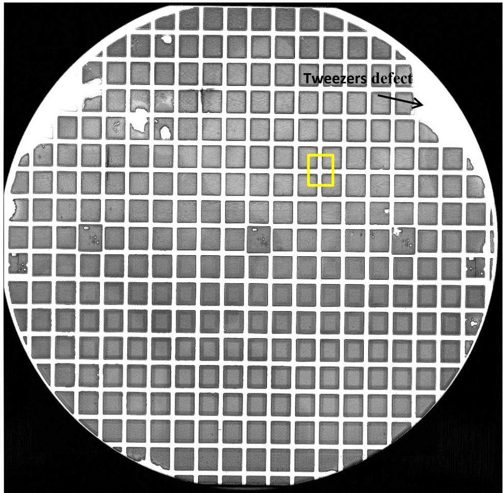
Figure 6.5. SAM image for full wafer solid-state bonding of a-Si with SC1 and HF cleaning prior to bonding. The sample was bonded at 350°C for 20 min.
