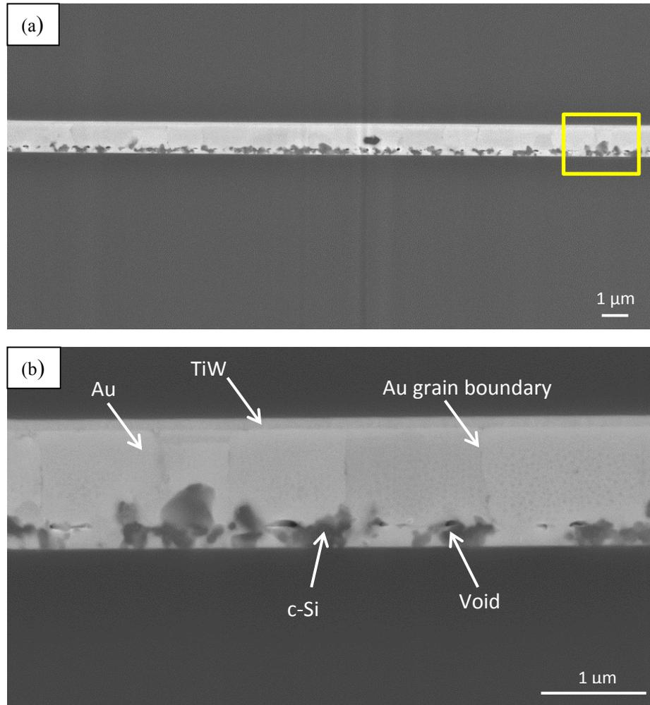
Figure 6.6. Microstructure of a-Si bonded sample bonded at 350°C for 20 min. (a) Low magnification and (b) higher magnification images of the rectangle area in Figure 6.5.
