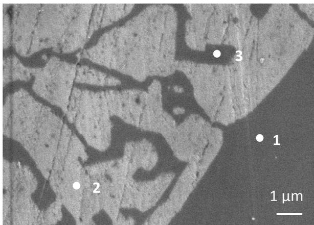
Figure 5.18. SEM SE cross section image taken at 1 kV from the crater area in the c-Si sample bonded at 400°C for 30 min (sample 1).
