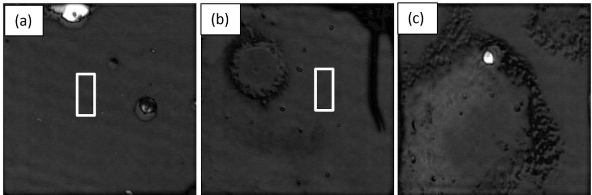
Figure 5.31. SAM images of three of five solid-state diffusion bonded Au/c-Si samples (heated to 350°C for 20 min).
