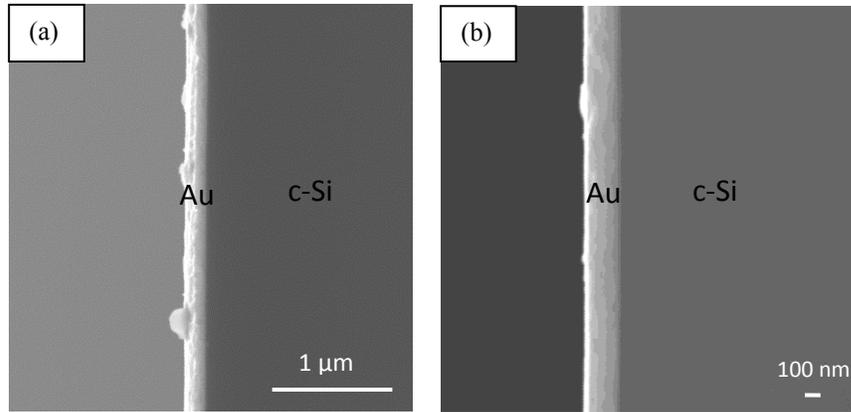
Figure 4.2. SEM SE images of cleaved cross sections for as-deposited Au/Ti/c-Si diffusion couple: (a) low magnification image and (b) higher magnification image. The sample was stored for 2 weeks at room temperature prior to imaging.
