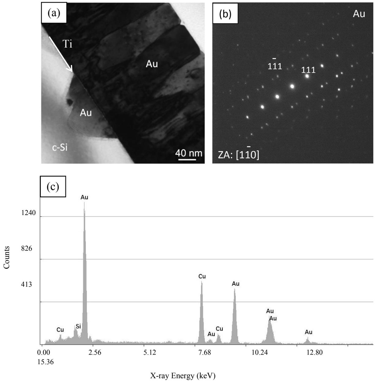
Figure 4.14. (a) TEM BF image, (b) SAD pattern and (c) EDX spectrum from the crater area of a Au/Ti/c-Si sample annealed at 350°C for 30 min.
