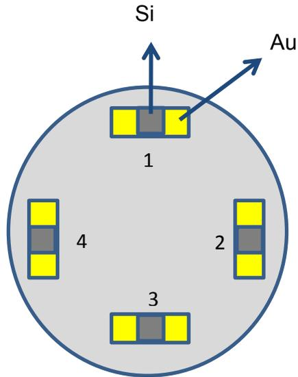
Figure 5.9. Four sample configuration used on the chuck in order to improve pressure uniformity.
