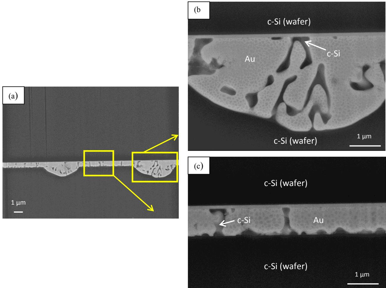
Figure 6.9. SEM SE cross section images of c-Si sample eutectic bonded at 350°C for 20 min taken from the region indicated in Figure 6.8. (a) Low magnification image, (b) high magnification image of the crater area and (c) high magnification image of non-crater area.
