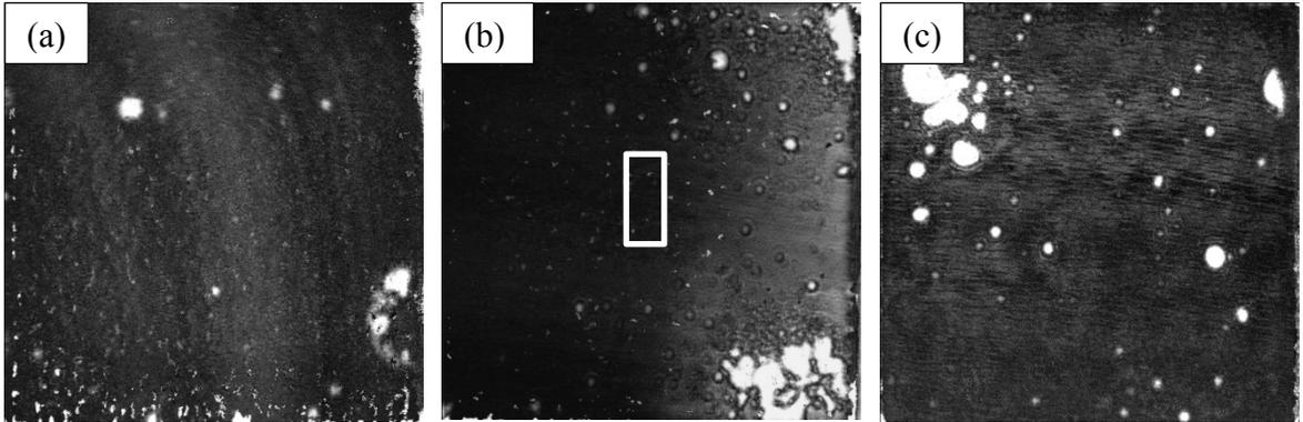
Figure 5.24. SAM images taken from three of the five c-Si/Au eutectic bonded samples (preheated at 350°C for 20 min and bonded at 400°C for 30 min).
