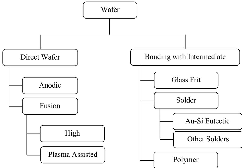
Figure 2.1. Classification of wafer bonding [10].
