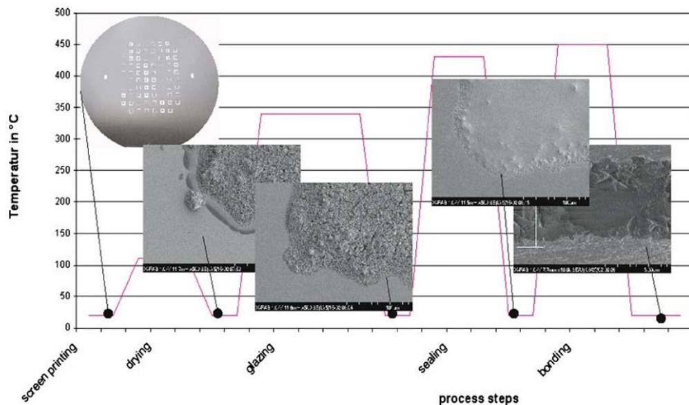
Figure 2.4. Thermal conditioning during glass-frit bonding [26].
