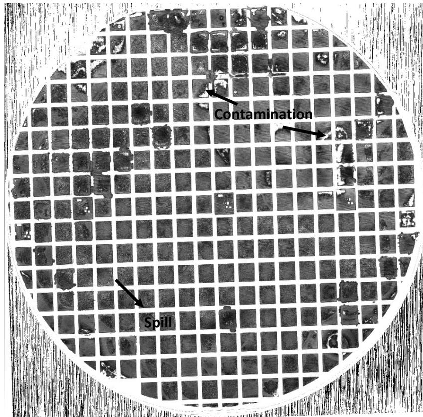
Figure 6.1. SAM results for full wafer eutectic bonding of a-Si with HF cleaning prior to bonding.
