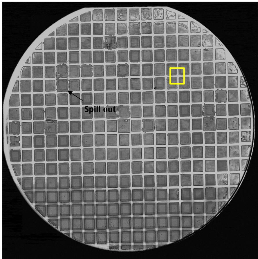
Figure 6.2. SAM image for full wafer eutectic bonding of a-Si with SC1 and HF cleaning prior to bonding. The sample was preheated to 350°C and then bonded at 400°C.
