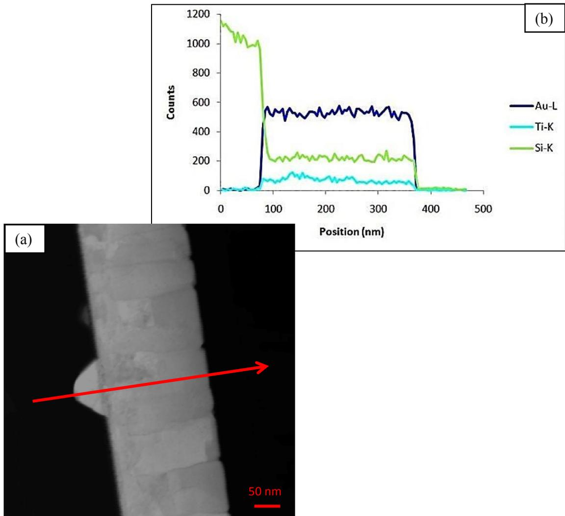
Figure 4.15. (a) STEM high angle annular dark-field (HAADF) image of a cross section specimen of the Au/Ti/c-Si sample annealed at 350°C for 30 min. (b) X-ray line scan across the interfacial region (indicated by the arrow in (a)).
