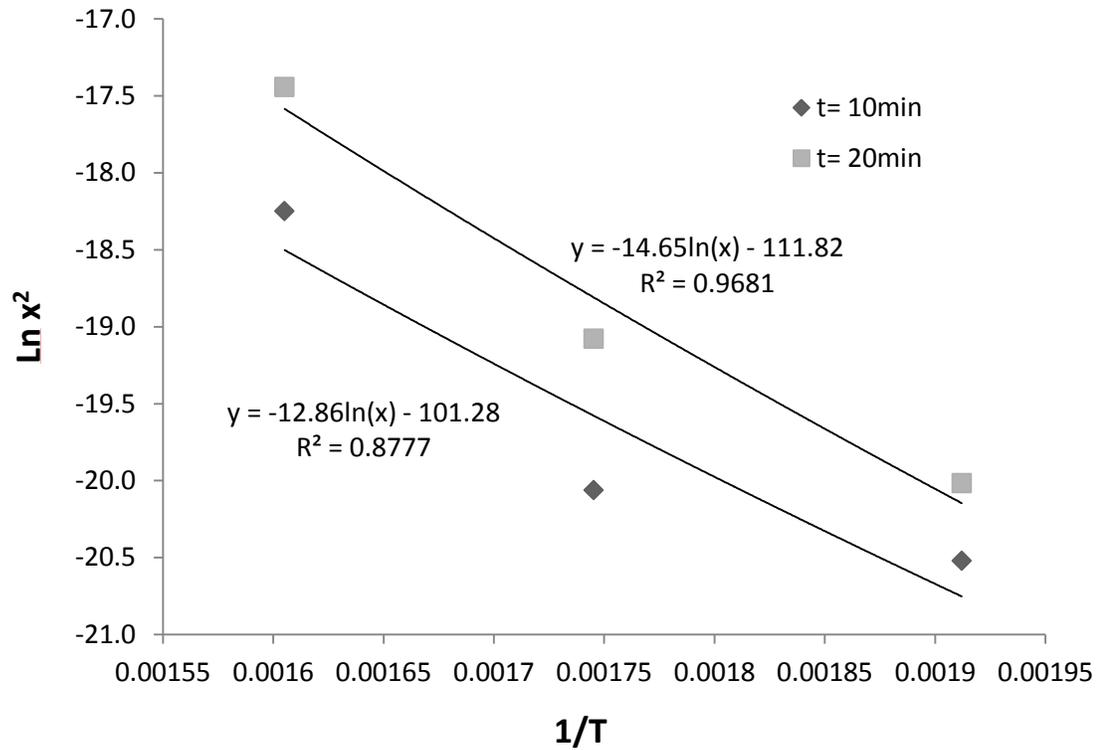
Figure 4.8. Plot of the natural logarithm of diffusion depth squared vs. inverse annealing temperature for a-Si diffusion couples annealed for 10 and 20 min.
