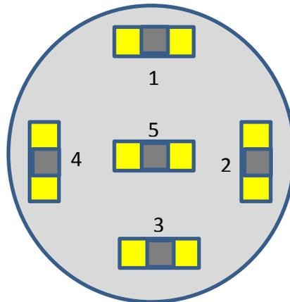
Figure 5.11. Five sample configuration used on the chuck to improve pressure uniformity.
