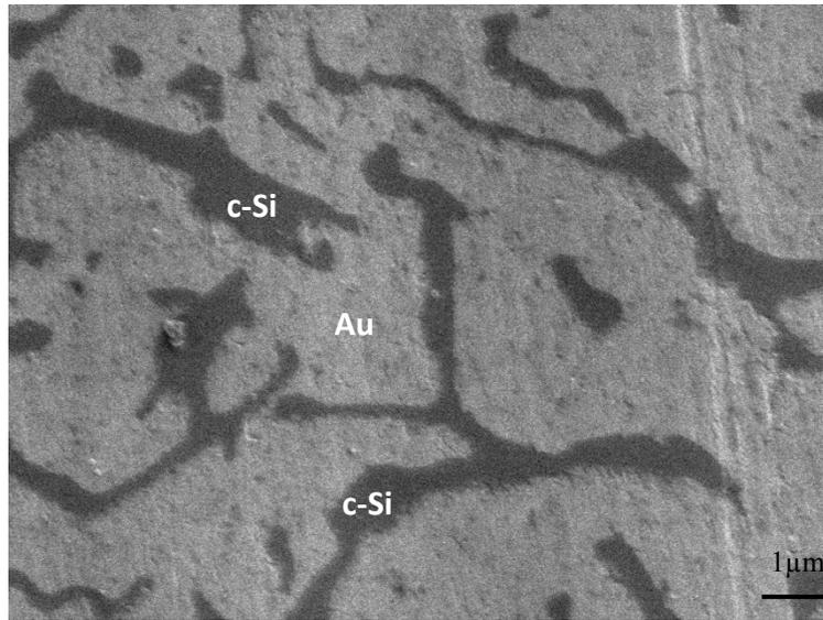
Figure 6.10. SEM SE cross section image (1 kV) of crater area in eutectic bonded c-Si sample (bonded at 350°C for 20 min).
