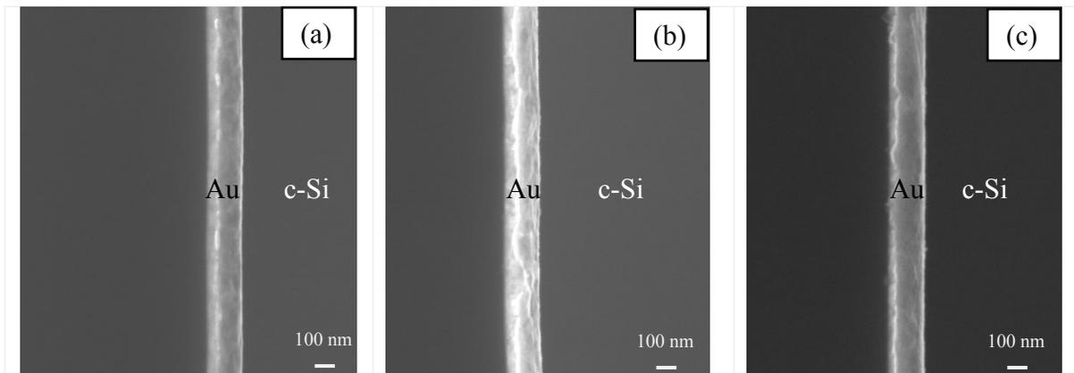
Figure 4.9. SEM SE images of cleaved cross sections for Au/c-Si diffusion couples annealed at 250°C for (a) 10 min, (b) 20 min and (c) 30 min.
