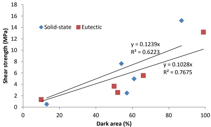
Figure 5.34. Shear strength vs. bonded area percentage for eutectic and solid-state bonded samples.
