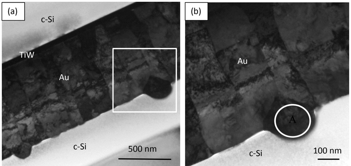
Figure 5.33. TEM BF images of FIB sample prepared from region indicated in Figure 5.31(a): (a) Low magnification image and (b) higher magnification image of region in (a); SAD pattern of Au particle is also shown.
