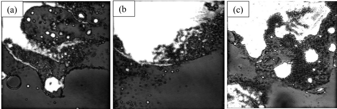
Figure 5.16. SAM images of three eutectic a-Si/Au bonded samples preheated at 350°C for 20 min and bonded at 400°C for 30 min. The sample locations on the chuck were location 1 as shown in Figure 5.11.
