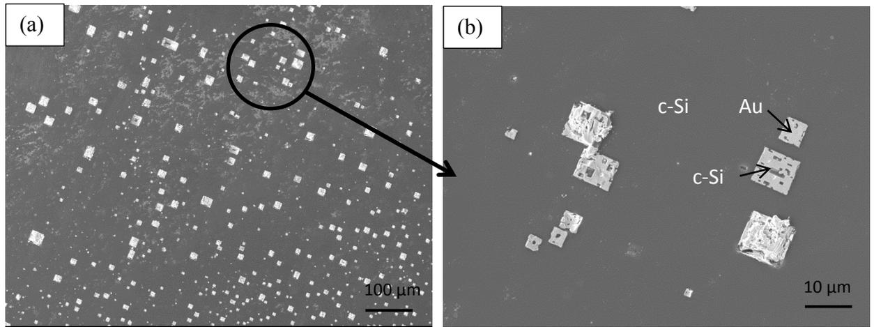
Figure 5.21. Plan view SEM SE images from detached Au/c-Si pieces bonded at 400°C for 30 min (sample 2): (a) low magnification and (b) high magnification.
