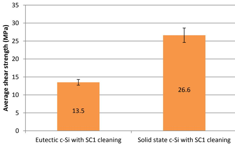
Figure 6.19. Shear strength comparison of a-Si eutectic bonded sample with solid-state bonded samples.
