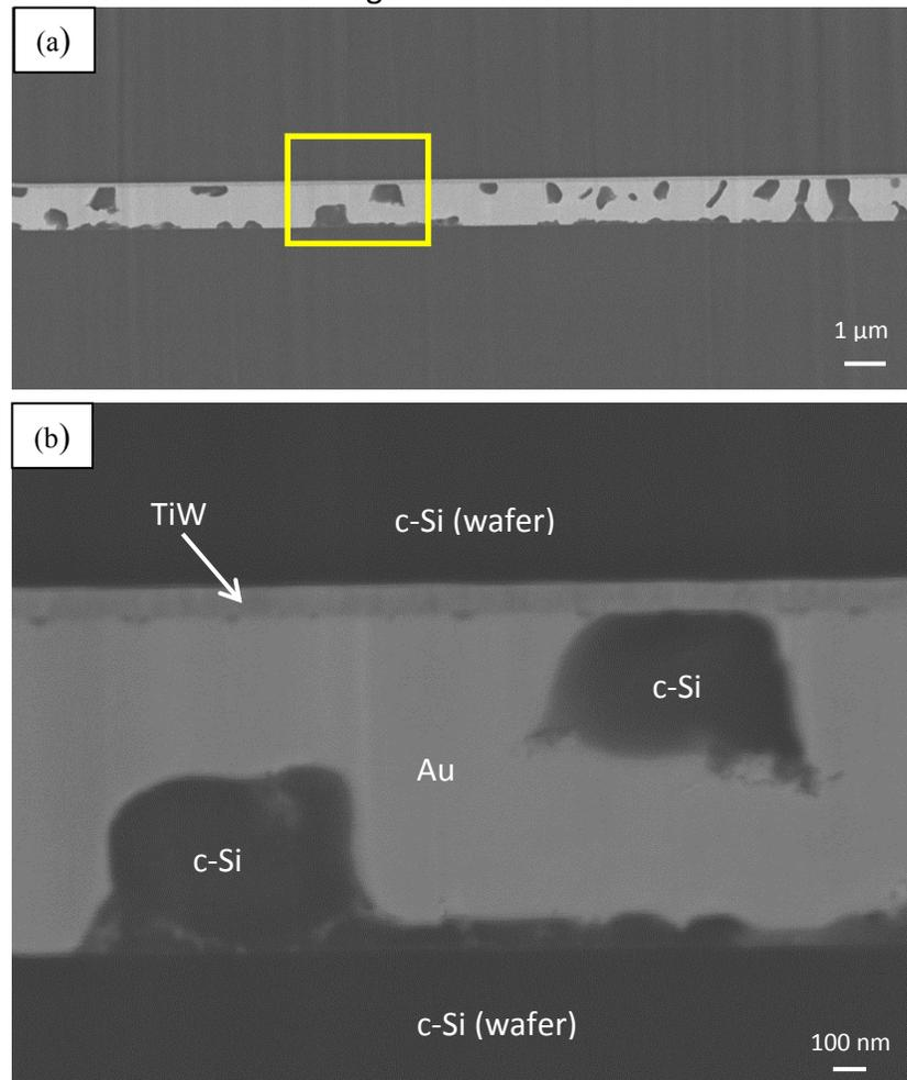
Figure 6.3. Microstructure of a-Si bonded sample preheated at 350°C for 20 min and bonded at 400°C for 15 min. (a) Low magnification and (b) higher magnification images of the rectangle area in Figure 6.2.
