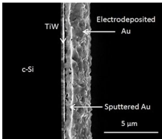
Figure 5.1. SEM BSE cleaved cross section image of Si/TiW/sputtered Au/electrodeposited Au layers.
