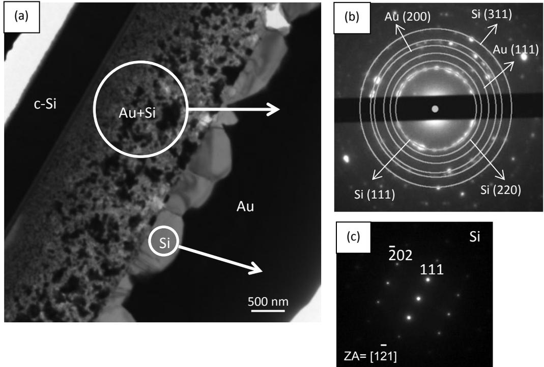
Figure 4.6. a) TEM BF image, b) SAD pattern of the Au-Si intermixed region and c) SAD pattern from the Si grain indicated in (a) for the Au/a-Si diffusion couple annealed at 350°C for 30 min.
