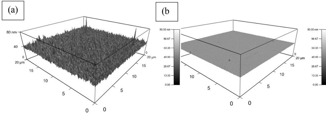
Figure 5.7. AFM surface roughness measurement of a-Si deposited by (a) PECVD and (b) LPCVD methods.
