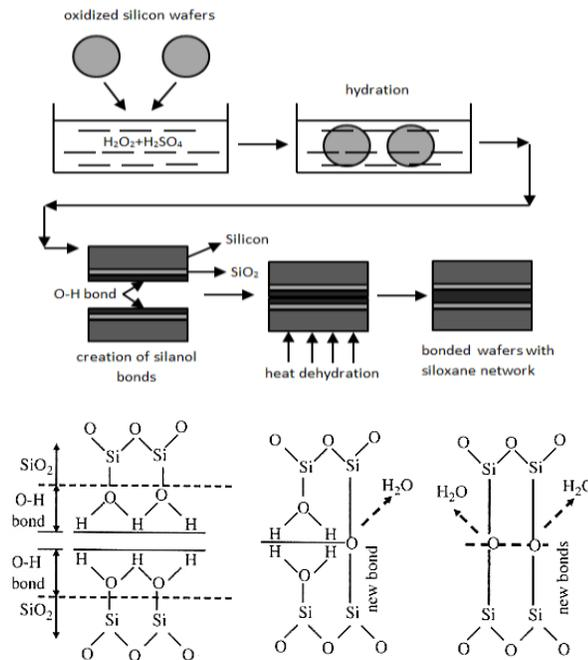
Figure 2.2. Si direct bonding by hydration [17].
