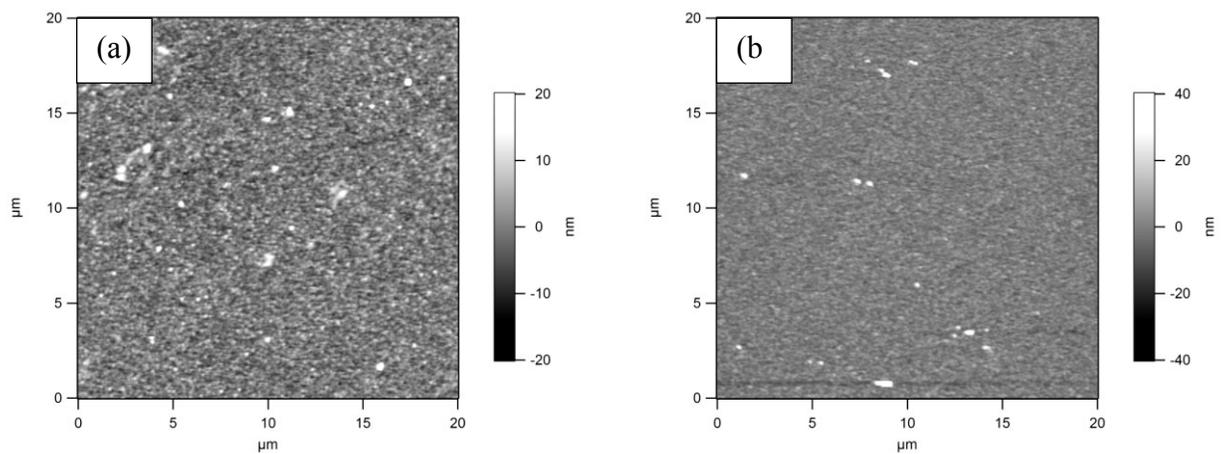
Figure 5.6. AFM plan view images of a-Si layer deposited by (a) PECVD and (b) LPCVD methods.
