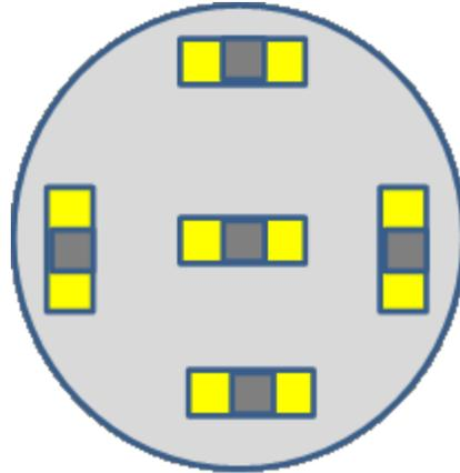
Figure 3.4. Five sample configuration used on the chuck in order to improve pressure uniformity.
