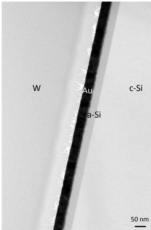
Figure 7.2. BF TEM cross section image of FIB polished Au/a-Si/c-Si sample after reaching 250°C in 600s.
