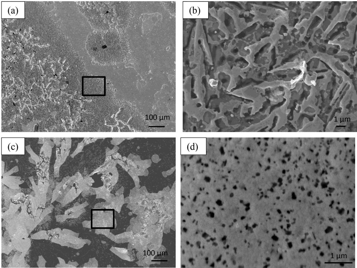
Figure 5.4. SEM SE plan view images of sample 2 (a-Si bonded at 400°C) pieces after dicing. The Au side: (a) low magnification image and (b) high magnification of the area indicated in (a). The Si side: (c) low magnification image and (d) high magnification of the area indicated in (c).
