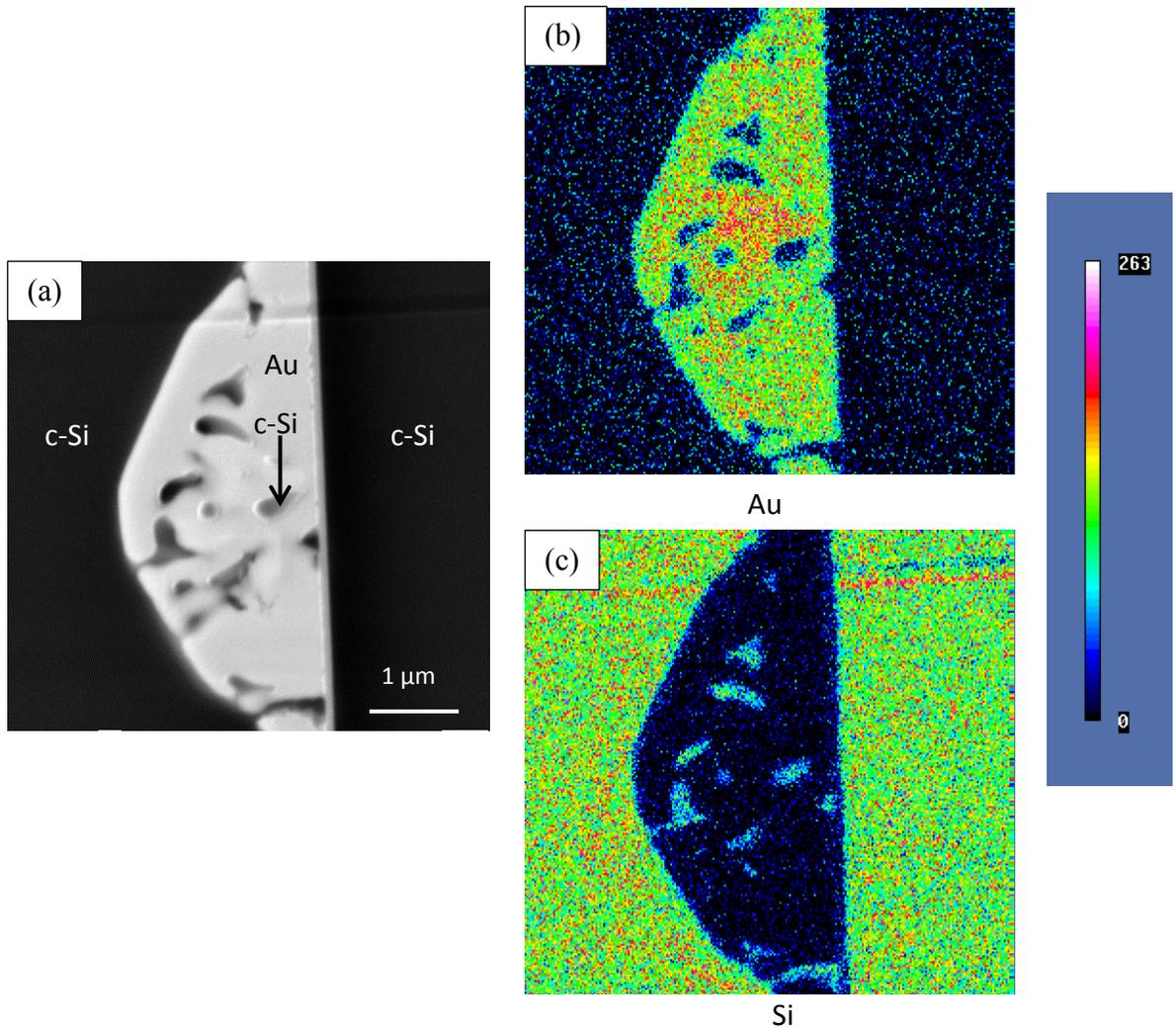
Figure 6.11. AES maps taken from the (a) SE SEM cross section image of the sample bonded at 350°C for 20 min. (b) Au map and (c) Si map of a crater area in the c-Si eutectic bonded sample.
