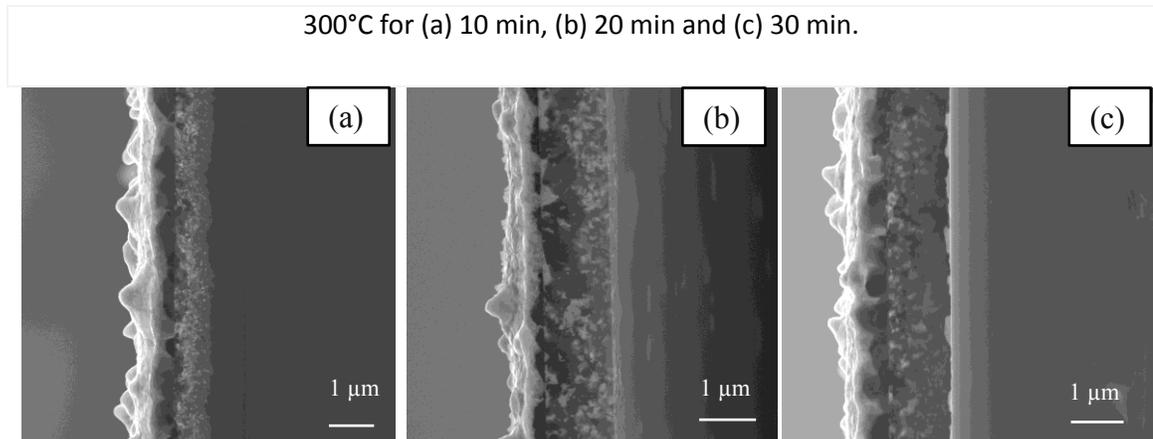
Figure 4.5. SEM SE images of cleaved cross sections for Au/a-Si diffusion couples annealed at 350°C for (a) 10 min, (b) 20 min and (c) 30 min.
