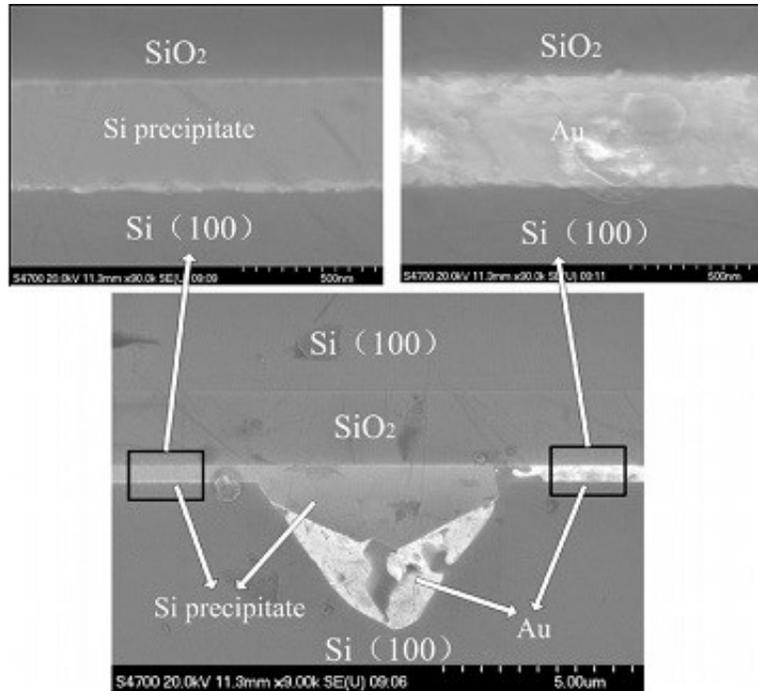
Figure 2.6. Cross-sectional SEM image of an Au/c-Si bond structure. The bond interface consists of crater and non-crater regions and these regions are filled with Si precipitates or Au [48].
