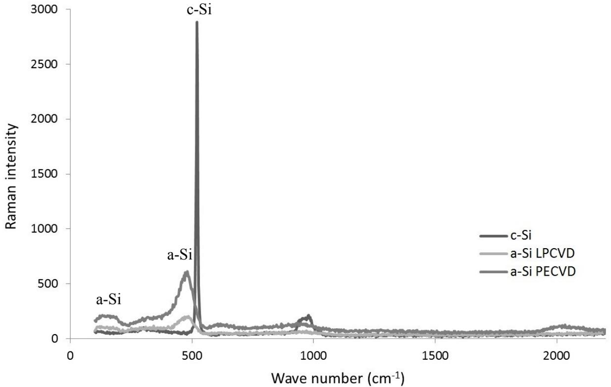
Figure 5.8. Raman spectra obtained from c-Si, a-Si deposited by LPCVD and a-Si deposited by PECVD. Laser power: 4.32 mW; exposure time: 10 s, laser wavelength: 514 nm.
