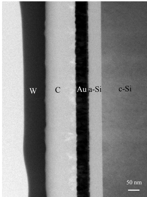
Figure 7.5. BF TEM cross section image of FIB polished Au/a-Si/c-Si sample before annealing.
