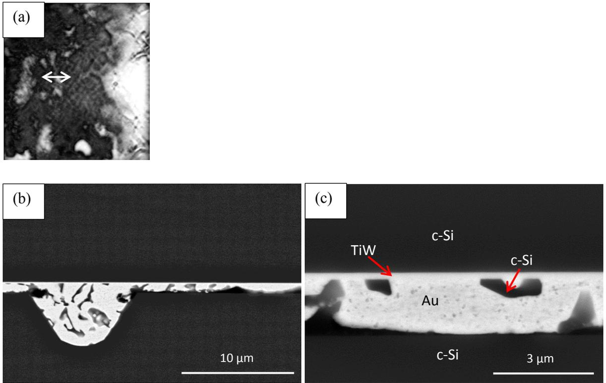
Figure 5.17. Cross section BSE SEM images (25 kV) from (b) crater and (c) non-crater area in c-Si sample preheated at 350°C for 20 min and bonded at 400°C for 30 min. The images were taken from the region indicated by the line shown in the SAM image (a) (sample 1).
