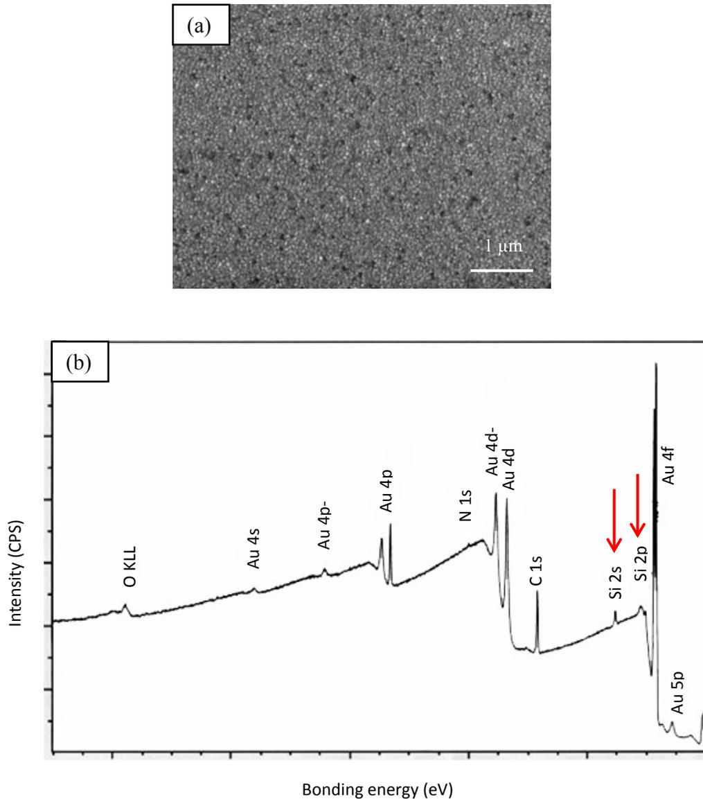
Figure 4.16. (a) SEM image from an as deposited Au surface for the Au/Ti/c-Si sample and (b) XPS spectrum from the Au surface showing the presence of Si on the Au surface. No Ti was detected on the surface.
