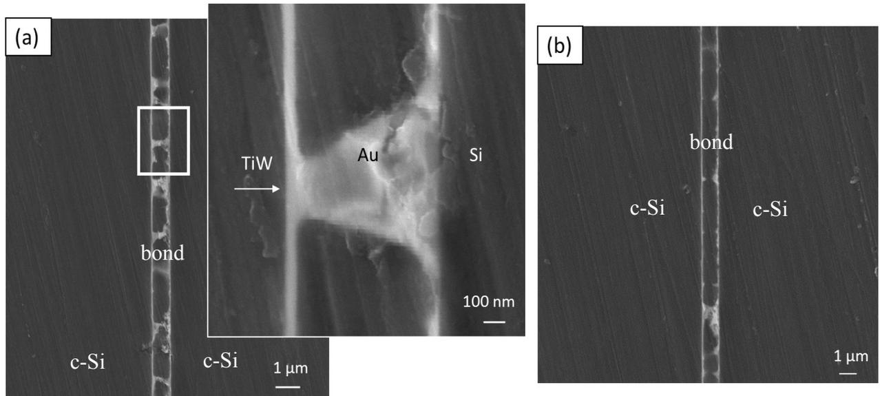
Figure 5.13. SEM SE images of cleaved cross sections of sample 2 in Figure 5.12. (a) Region shown by white rectangle and (b) region shown by black rectangle in Figure 5.12.
