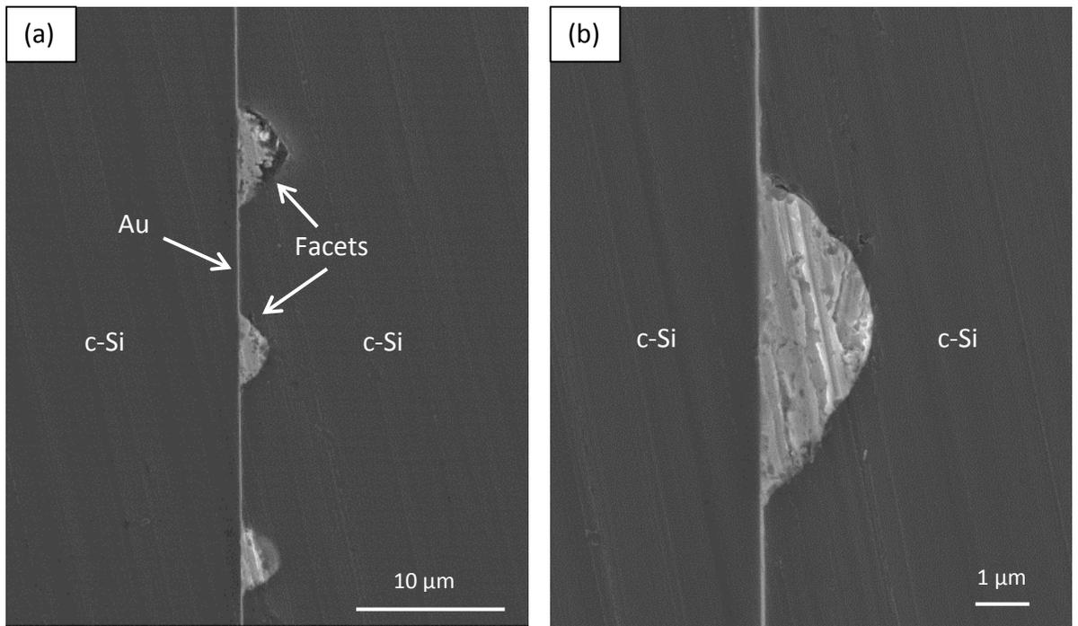
Figure 5.25. SEM SE images of cleaved Au/c-Si eutectic bonded sample: (a) low magnification image and (b) higher magnification image.
