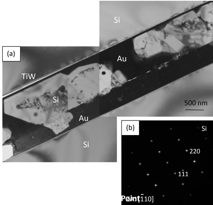
Figure 5.30. (a) TEM BF image of FIB sample prepared from the region indicated in Figure 5.28(c). (b) SAD pattern from one of the Si grains.
