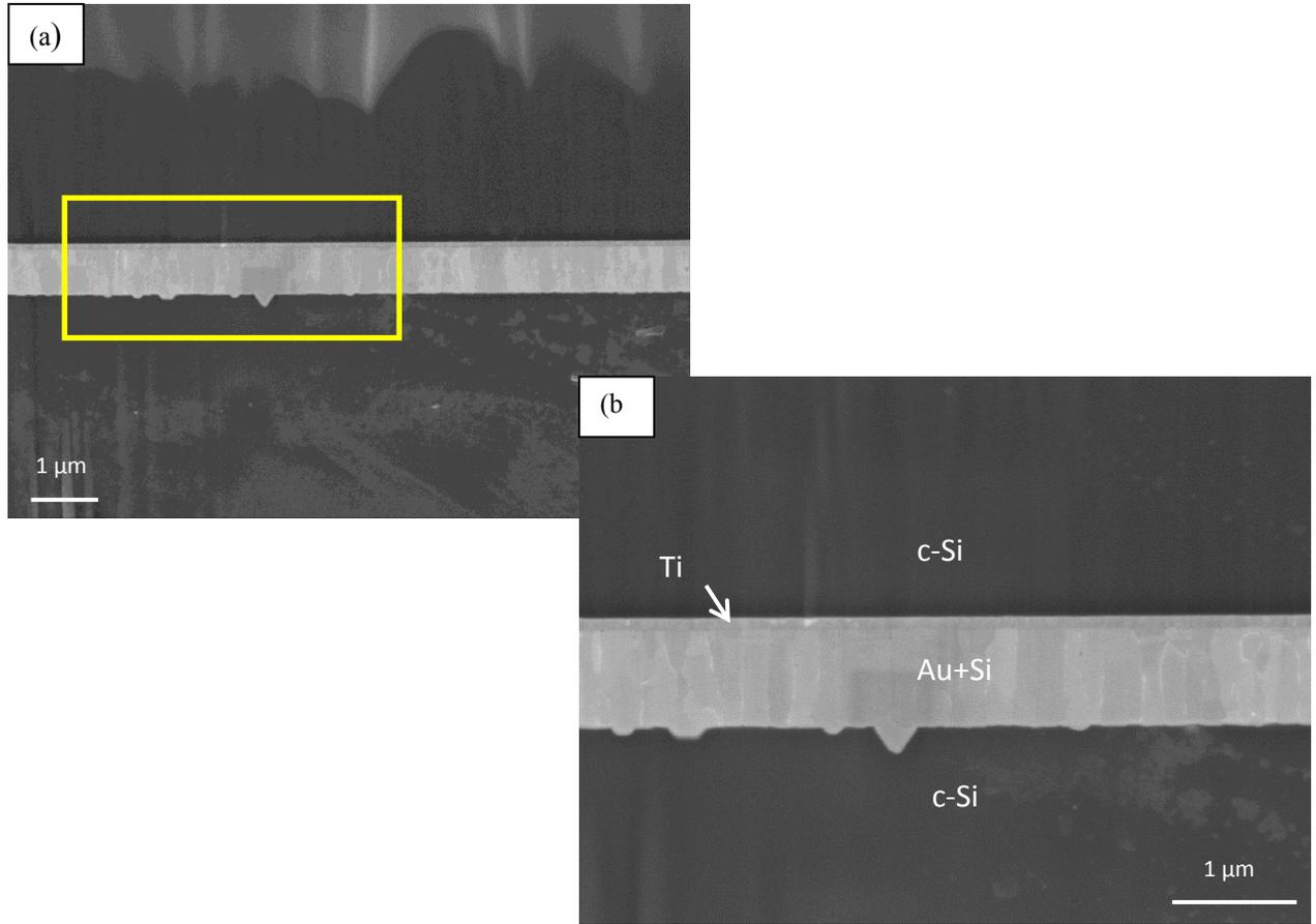
Figure 6.15. SEM SE cross section images of solid-state c-Si bonded sample region shown in Figure 6.14, bonded at 350°C for 20 min. (a) Low magnification image and (b) higher magnification image of the rectangle area in (a).
