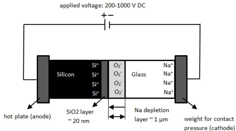
Figure 2.3. Schematic image of Si to glass bonding process [17].
