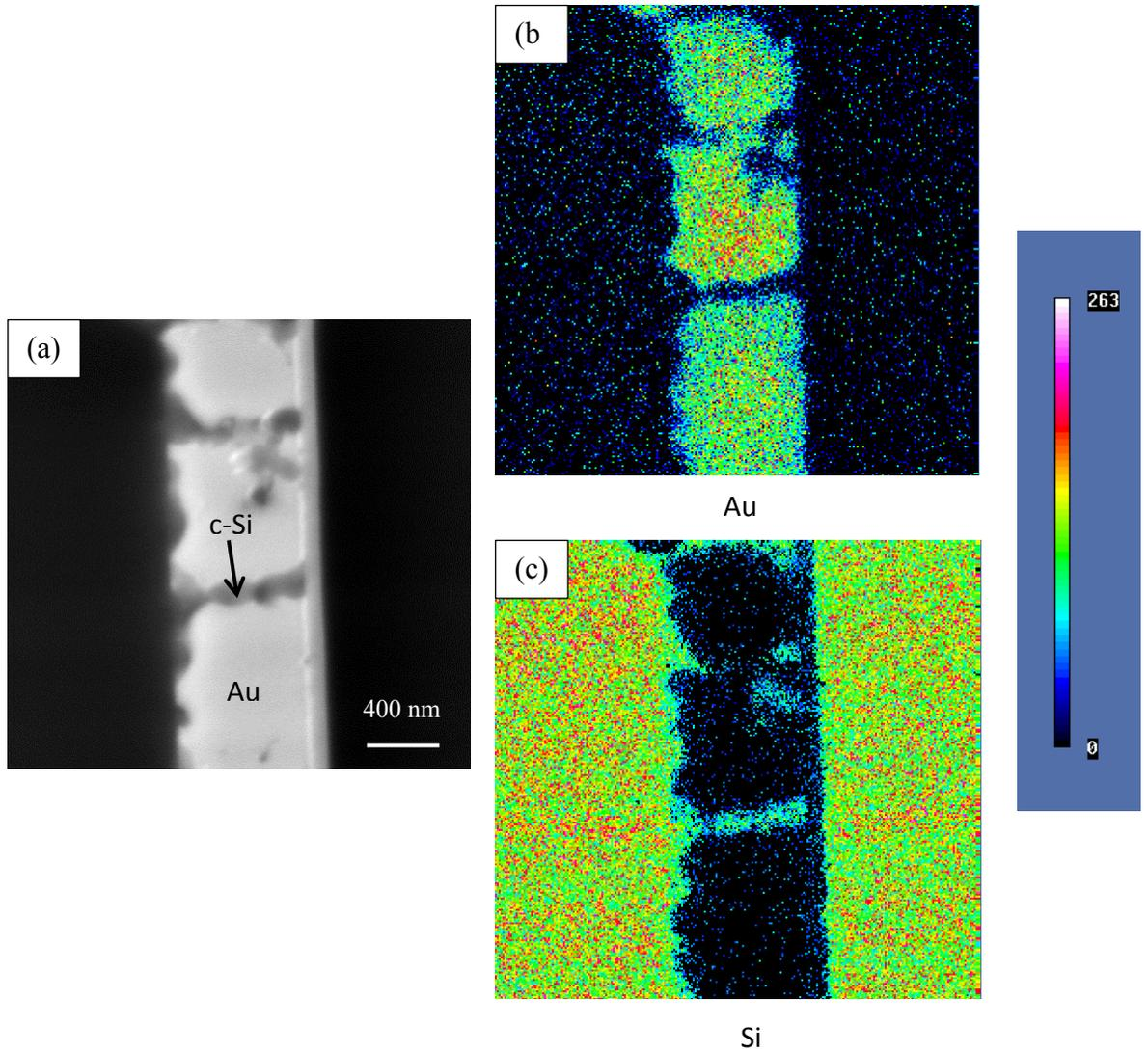
Figure 6.12. AES map taken from the (a) SE SEM cross section image of the sample bonded at 350°C for 20 min. (b) Au map and (c) Si map of a non-crater area in the c-Si eutectic bonded sample.
