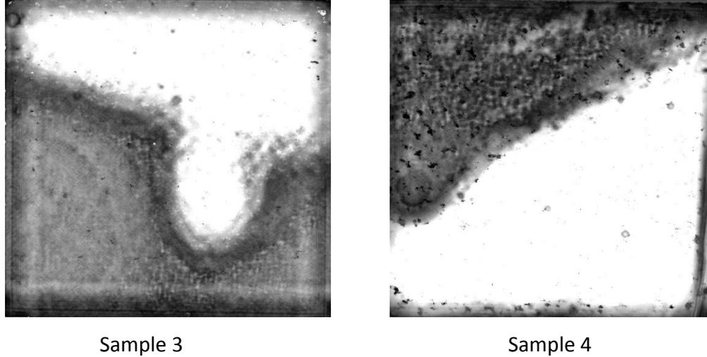
Figure 5.10. SAM results for the four sample configuration (LPCVD a-Si) shown in Figure 5.9.
