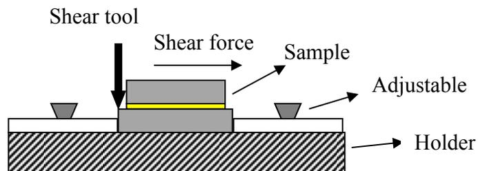
Figure 3.1. Schematic of the shear test tool set up (side view).
