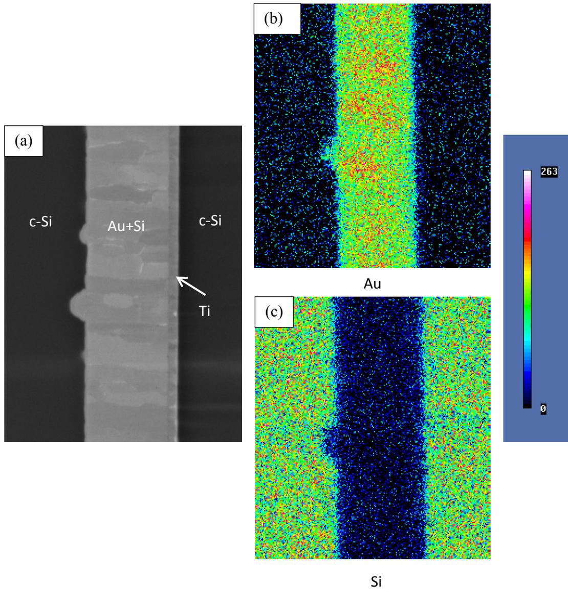
Figure 6.16. AES map taken from the (a) SE SEM cross section image. (b) Au map and (c) Si map of c-Si solid-state bonded sample.
