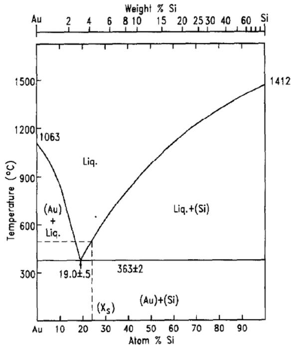
Figure 2.5. Au-Si phase diagram [46].
