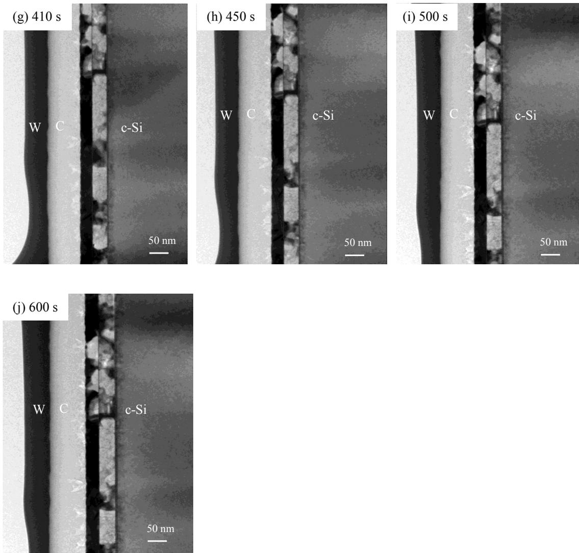
Figure 7.6. BF cross section TEM images of Au/a-Si sample during pre-heating to 300°C at (a) 300 s, (b) 350 s, (c) 360 s, (d) 380 s, (e) 390 s, (f) 400 s, (g) 410 s, (h) 450 s, (i) 500 s and (j) 600 s.
