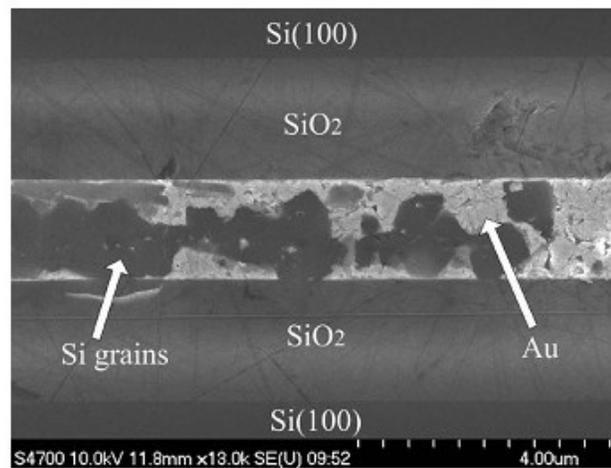
Figure 2.9. Cross-sectional SEM image of Au/a-Si bond [48].
