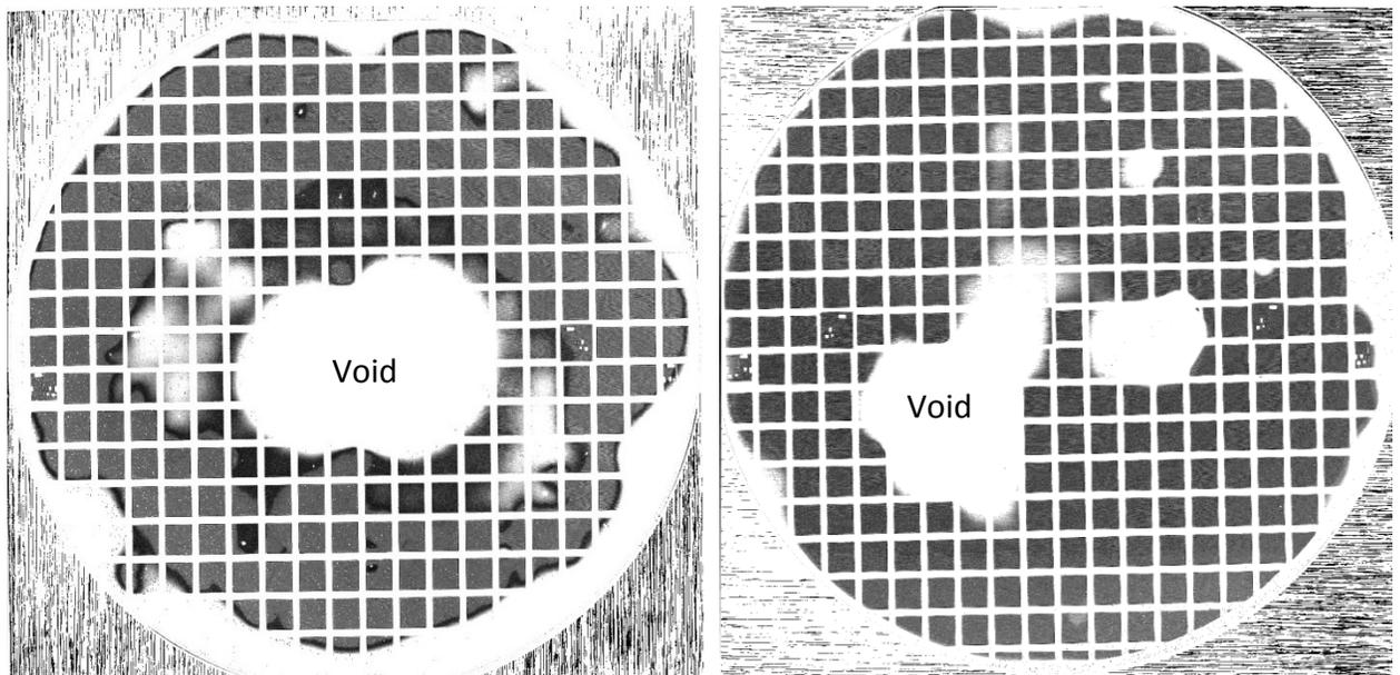
Figure 6.13. SAM images of c-Si solid state pairs bonded at 350°C for 20 min s. The bond test was repeated at a pressure of 0.06 MPa.
