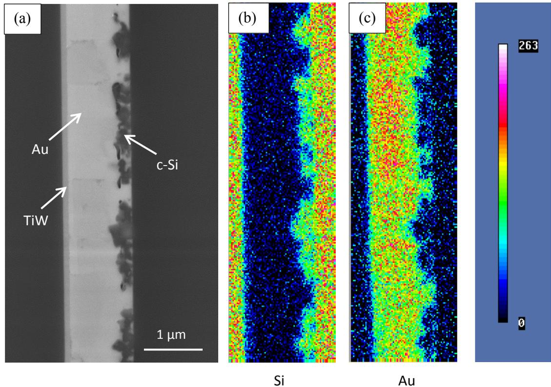
Figure 6.7. AES maps taken from the (a) SE SEM cross section image. (b) Si map and (c) Au map of a-Si solid-state bonded sample bonded at 350°C for 20min.
