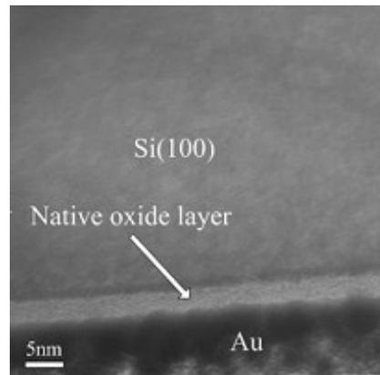
Figure 2.7. Cross-sectional TEM image of the Au/Si bonding structure. A thin native oxide is present at the bond interface of the non-crater regions [48].
