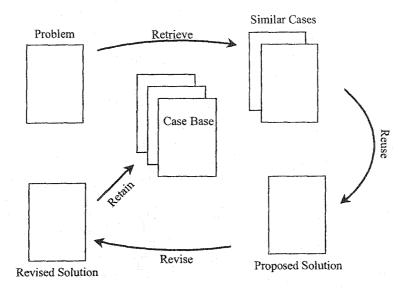
Figure A.1: The process of case based reasoning
