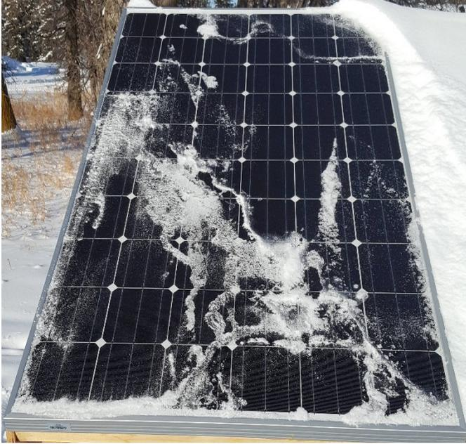
*Figure 4.4 Ice on framed PV panel resulting from large amounts existing snow accumulation melting (Event 7)*
