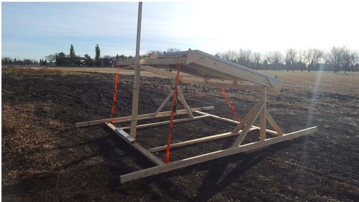
*Figure 3.2 View of the Experimental Setup Towards the South-East (frameless panel, pneumatic actuation, and instrumentation were not yet been installed)*
