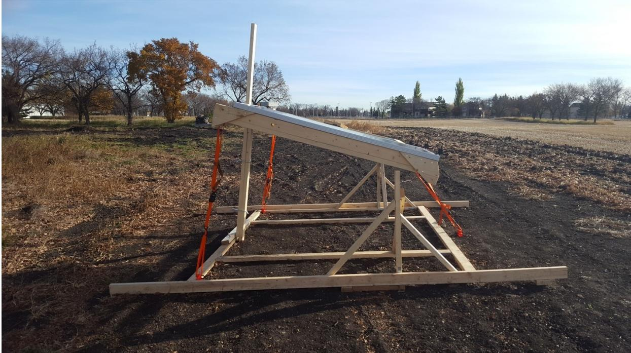
*Figure 3.3 View of the Experimental Setup Towards the East (frameless panel, pneumatic actuation, and instrumentation were not yet been installed)*
