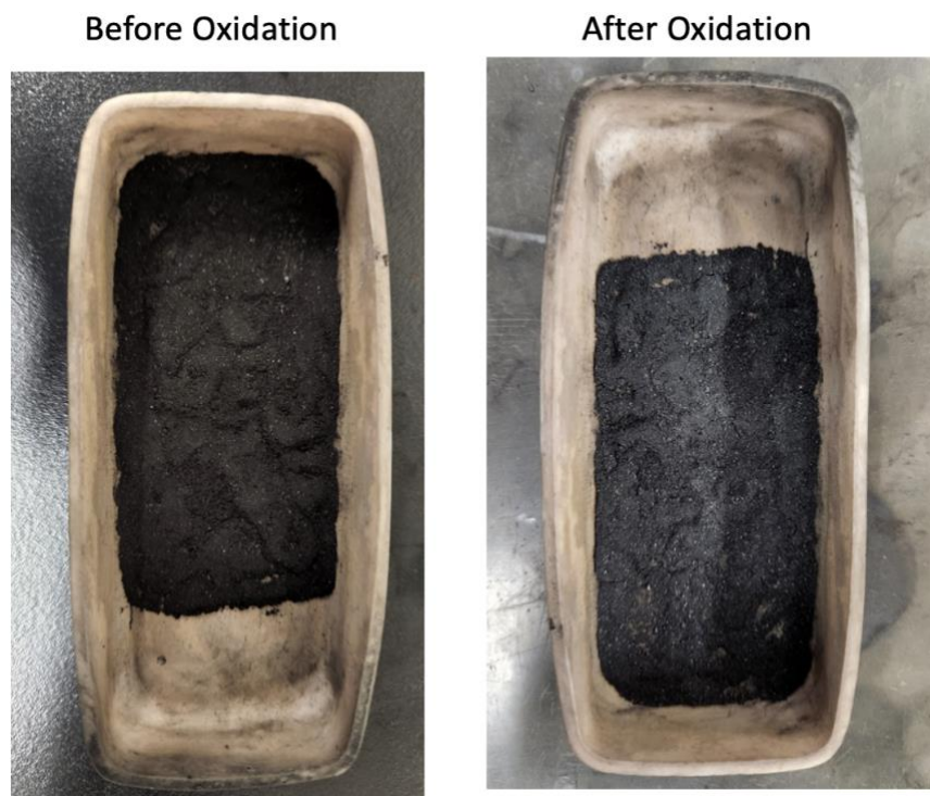
Figure 36: No melting observed under sufficient oxidative stabilization conditions
