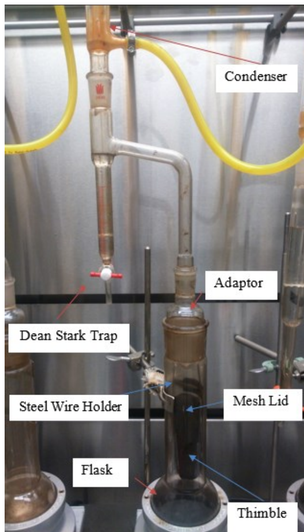
Figure 19. Dean Stark Apparatus
