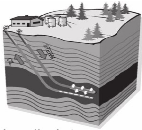
Figure 6. Schematic diagram of SAGD process. 7
