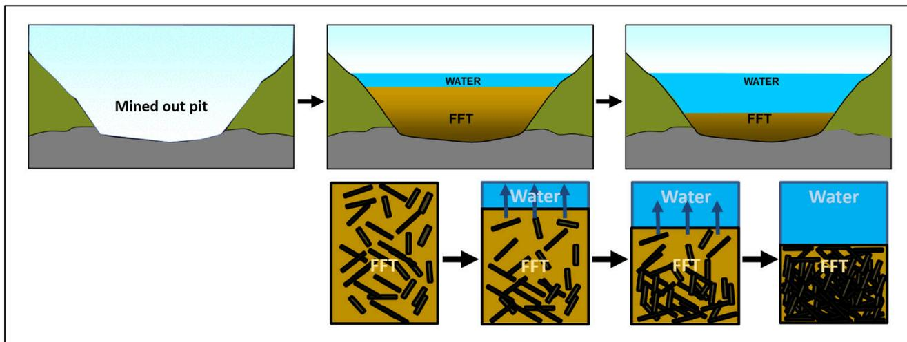
**Figure 3-2: Simplified Depiction of Water-Capped Tailings Settlement over Time (not to scale)**
