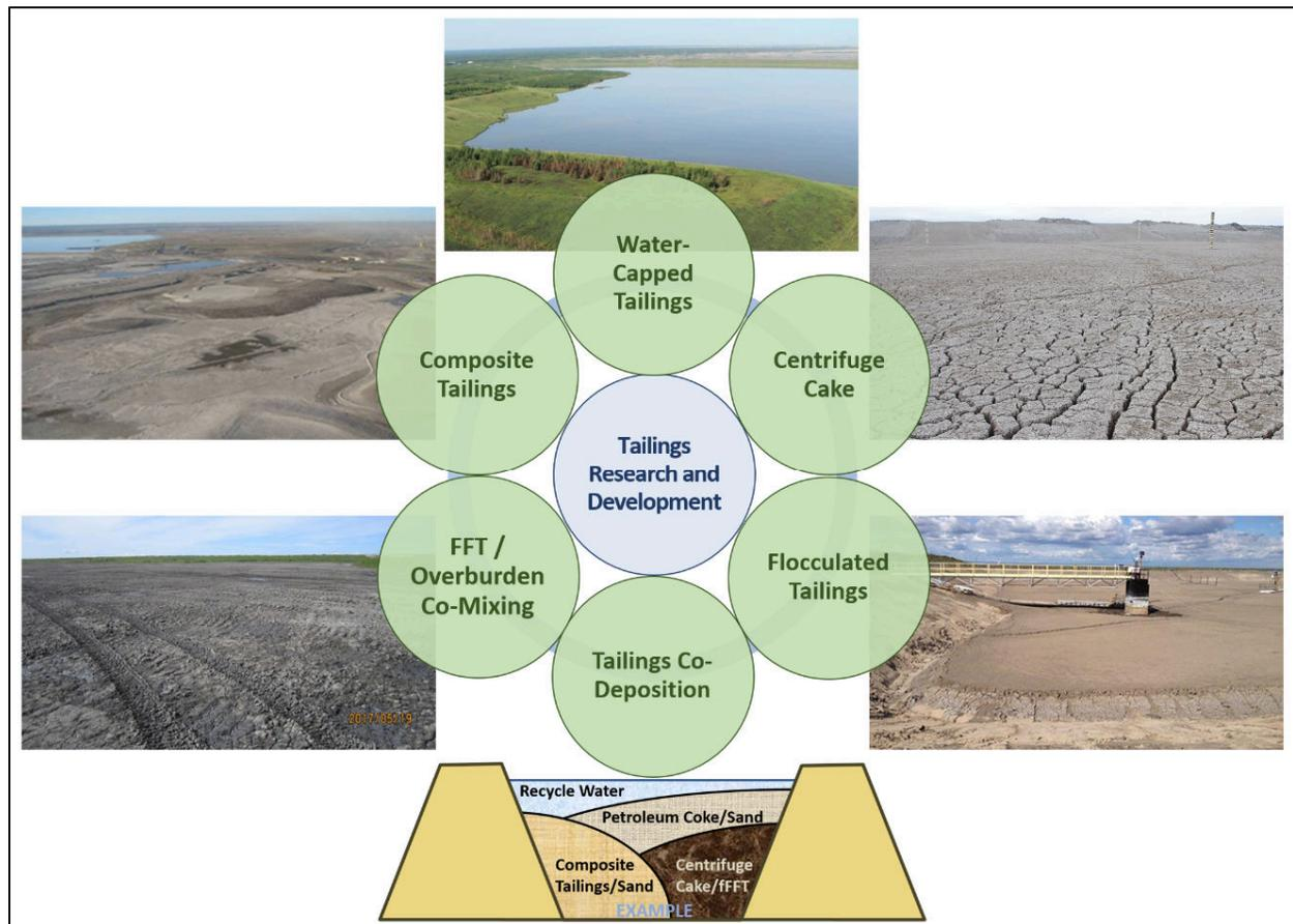
**Figure 3-1: Overview of Syncrude Fluid Tailings Treatment Technologies**
