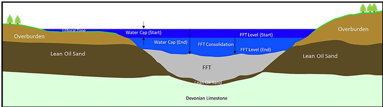
**Figure 3-3: Water-Capped Tailings Technology Schematic (not to scale)**
