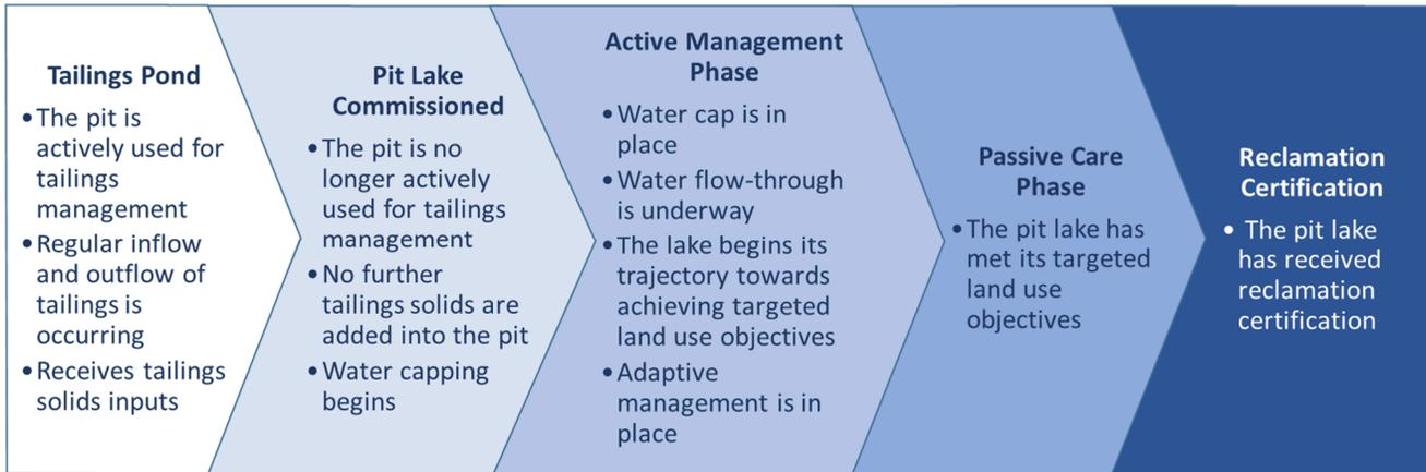
Figure 3-5: Conceptual Tailings Pond Progression into a Pit Lake
