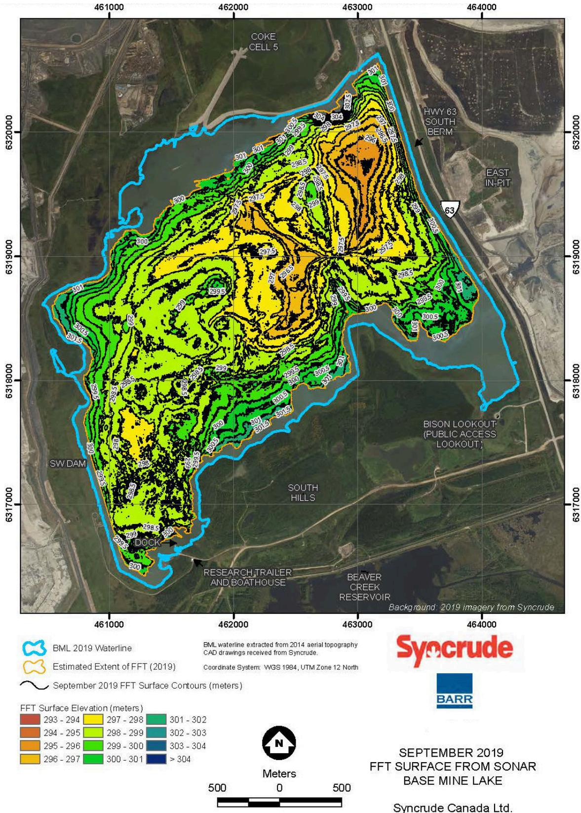
**Figure 5-1: Base Mine Lake FFT Surface from Sonar (September 2019)**
