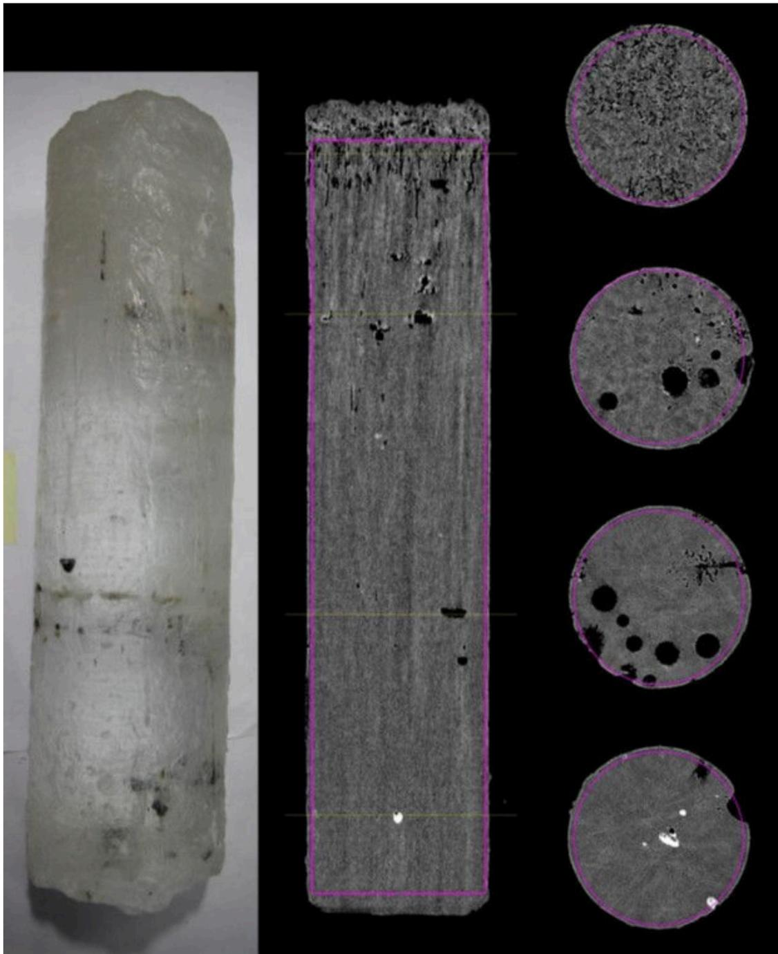
**Figure 5-10: Example Ice Core and the Imagery Produced from CT Scanning (including Cross-sections)<sup>7</sup>**
