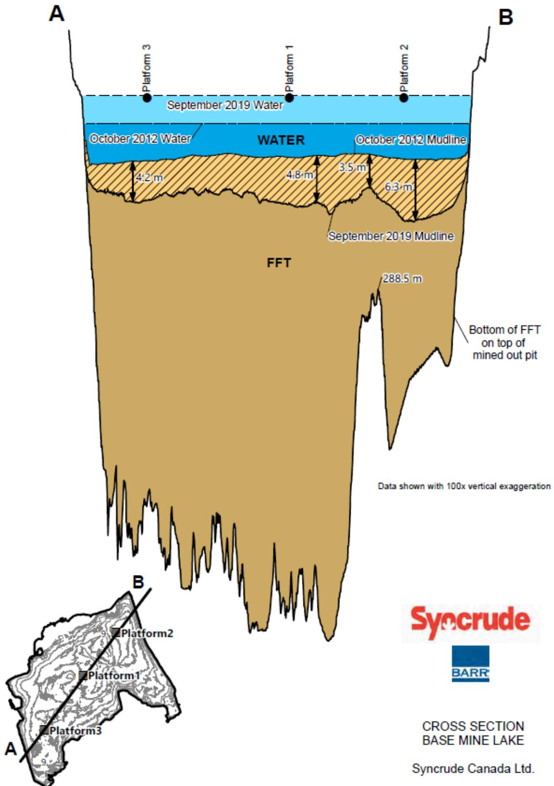
Figure 5-3: Cross-section of Base Mine Lake Showing Mudline Changes (2012-2019)
