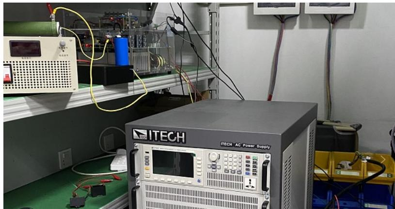
(b) Experimental setup for VSC impedance measurement
