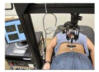
Fig. 1. Spinal stiffness testing by the mechanical indentation device.
