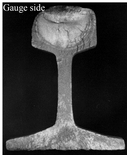
Figure 1.7 Transverse rail breaks due to internal defects [3]. Copyright 2009. Reproduced with permission from Elsevier.
