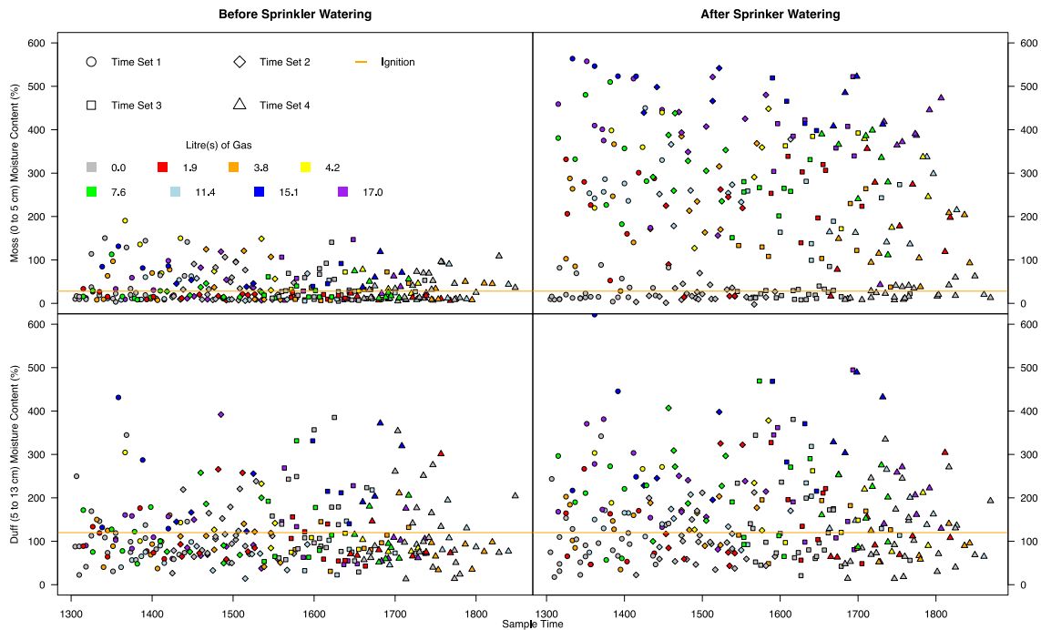
Figure 26. Moss and upper-duff moisture content levels before and after sprinkler-watering, a horizontal line indicates ignition probability threshold.
