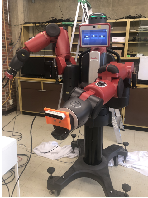
Figure 4.3: Experimental setup. The end-effector mounting plate holds a 3D-printed camera holder. An Intel RealSense D415 is mounted on the camera holder. The pose of the camera relative to the world frame is calculated using forward kinematics.
