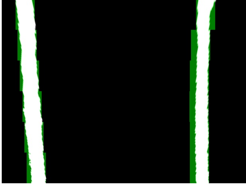
Figure 3.8: Sliding window search of the lane markings. Green blocks are each individual search window
