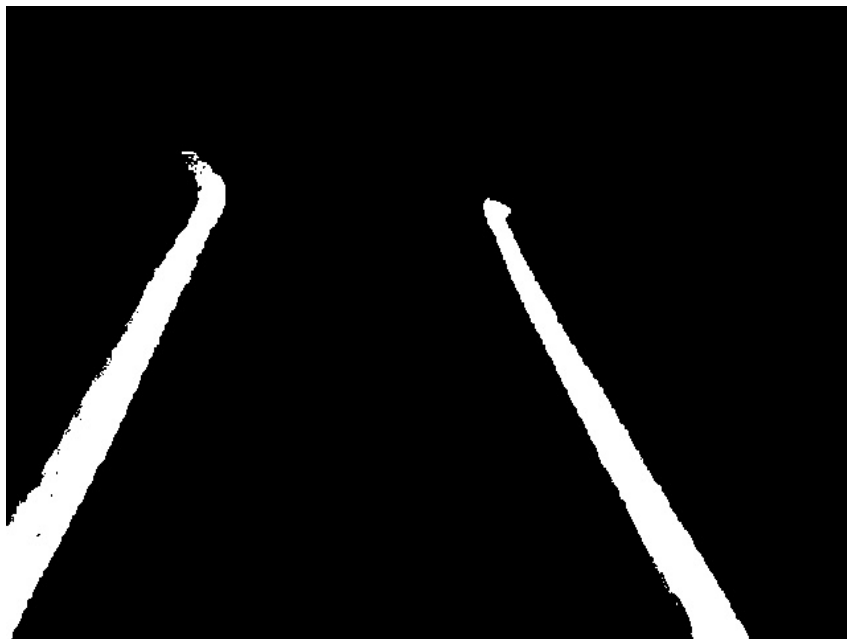
Figure 3.6: The binary image of lane masking after the HSV thresholds have been applied
