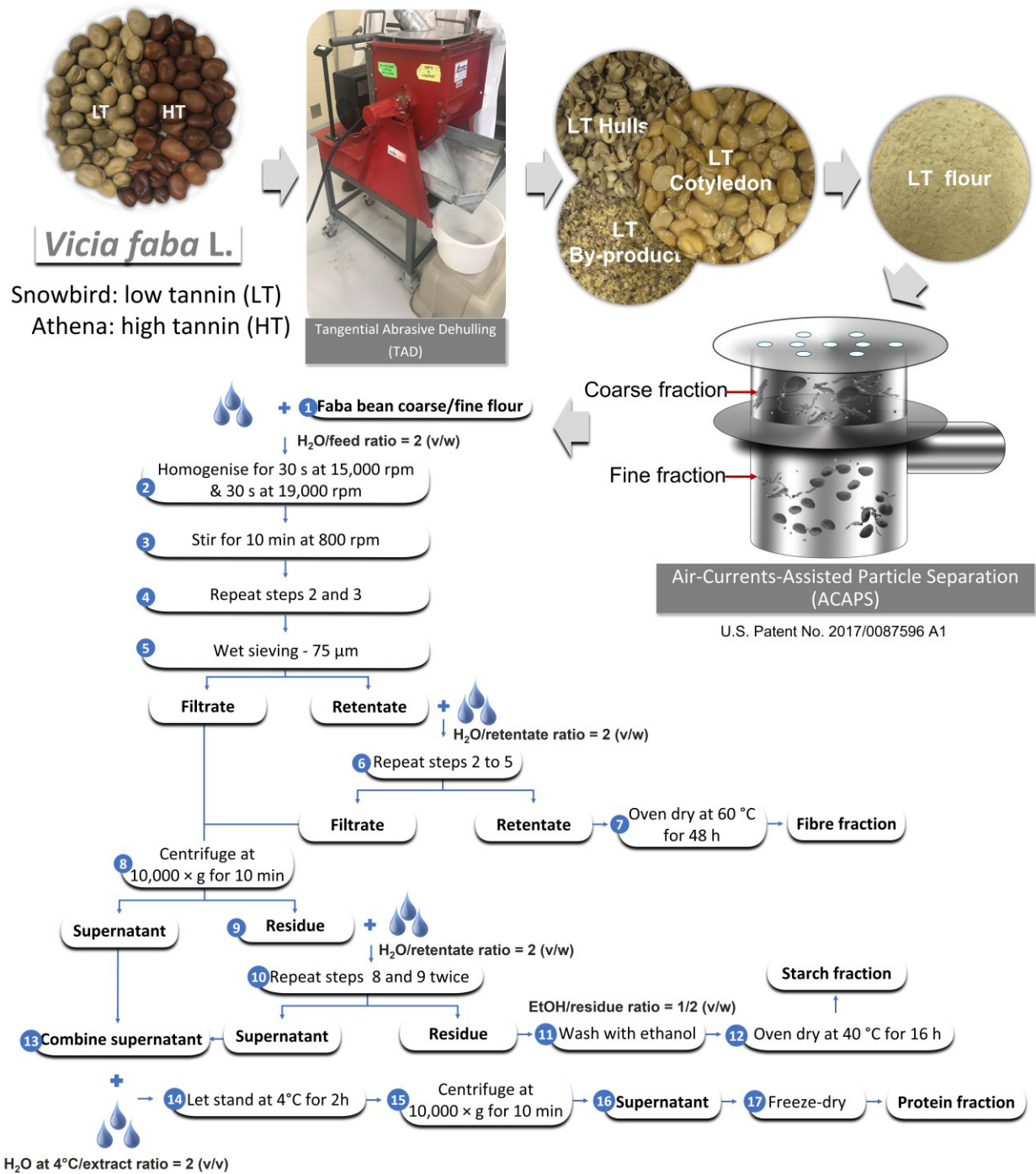
Fig. 5.2. Schematic overview of the air-currents-assisted particle separation (ACAPS) of faba beans followed by subsequent aqueous fractionation to isolate micellar proteins.
