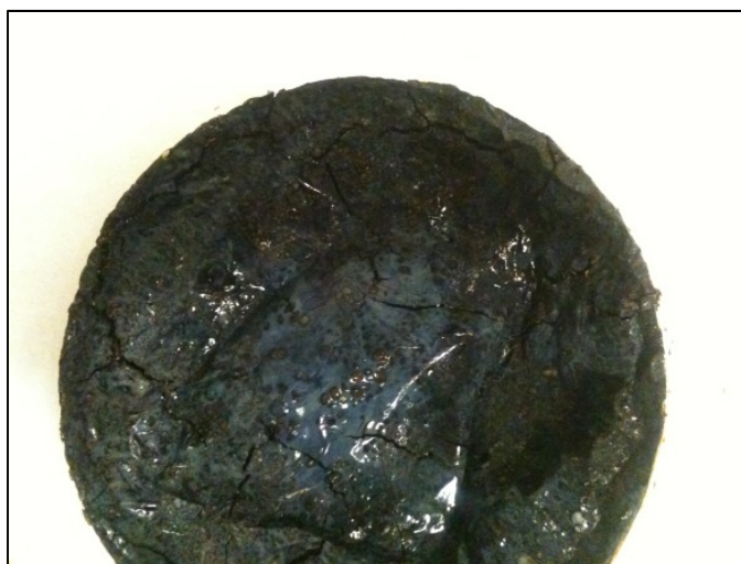
Figure 3.4. Top view of dried gel copper oxide precursor form Pechini method
