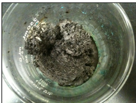
Figure 3.5. Plan view of the combustion product of oxidant to fuel ratio of 2.5 in
