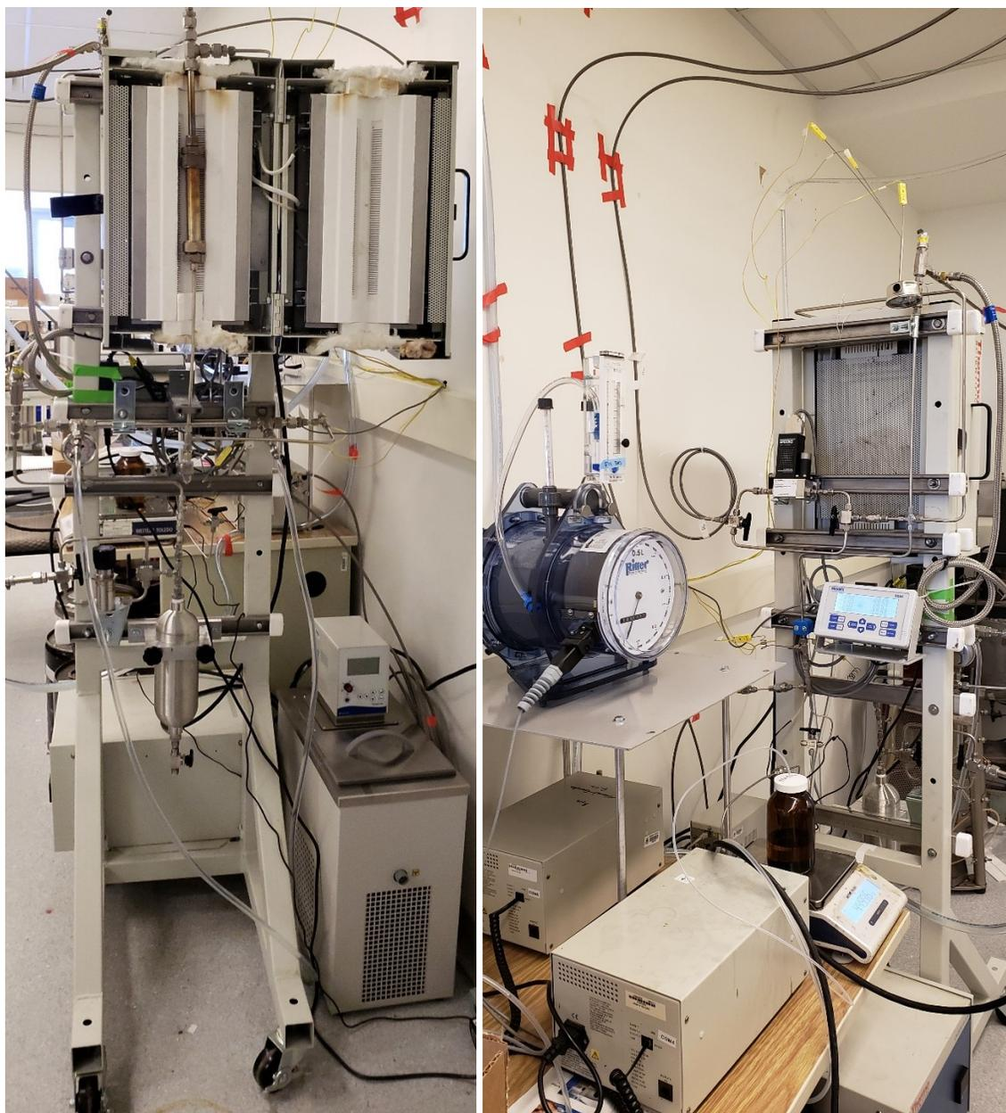
**Figure 6.3** Images of lab scale reactor which was designed, constructed and commissioned as part of this project
