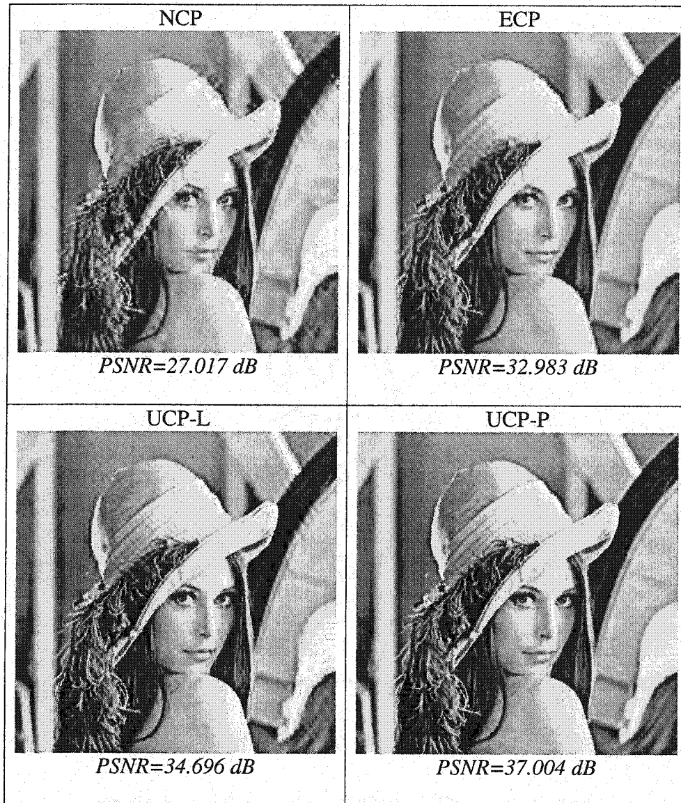
Figure 5.12. Visual results at 0.5bpp over a channel with \overline{SNR} = 20 dB for the gray-level Lena image. NCP is no channel protection. ECP is the equal channel protection technique. UCP-L is the unequal channel protection across the layers technique. UCP-P is the unequal channel protection across the packets technique.
