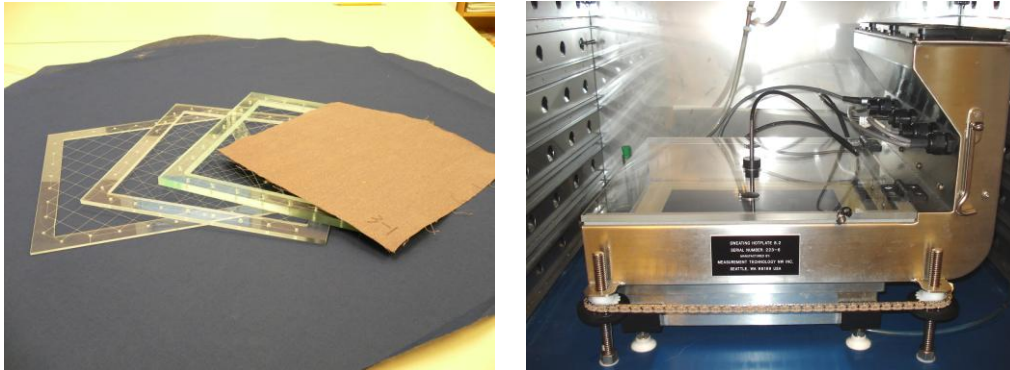
Figure 3-2 (a) Spacers (Air gap simulator), (b) Standard SGHP.
