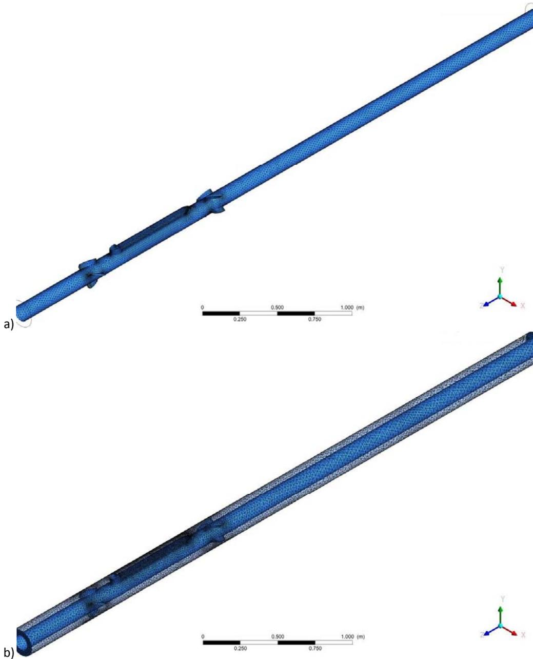
Figure 7.54 Mesh for the 3D model of (a) the novel sensor housing system and the casing conveyed with two sets of four flow deflector fins (Type-IV) each located at 127.0 mm down and up stream of sensor housing (b) within the 5.00 m of a borehole section.
