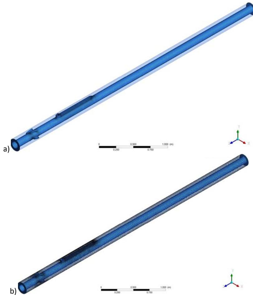
Figure 7.46 Mesh for the 3D model of (a) the novel sensor housing system and the casing conveyed with four flow deflector fins (Type-IV) located at 420.0 mm upstream of sensor housing (b) within the 5.00 m of a borehole section.
