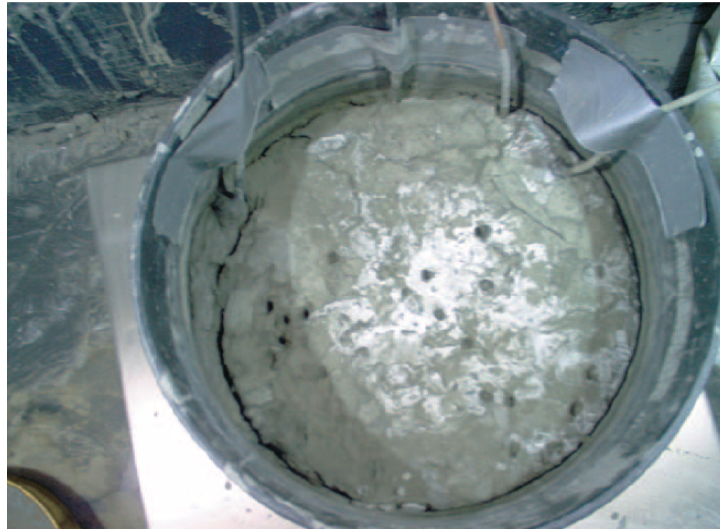
Figure 2.5 Formation of a white precipitate observed during water evaporation from paste tailings obtained in Bulyanhulu gold mine, Tanzania by Simms et al. (2007).
