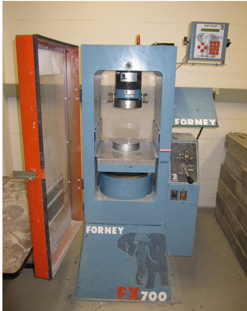
Figure 4.9 The compression testing machine at the University of Alberta used for loading the squeezer.
