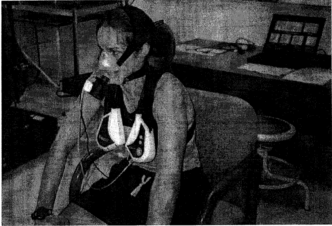
VmaxST system with chest strap, facemask, turbine, and laptop computer for data display.
